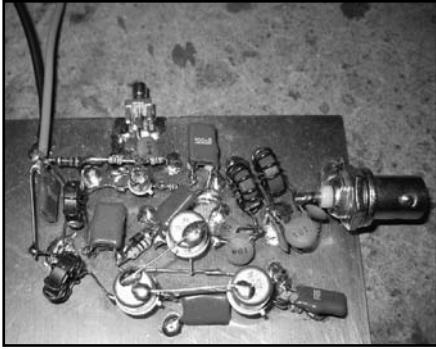
Figure 7 — This amplifier uses 2N2222 transistors to produce about 2 W of output power on the 40 m band.
