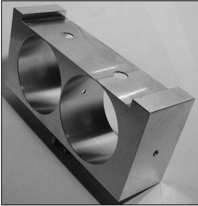
Figure 10 — This photo shows the dual TE 011 cavity filter.
