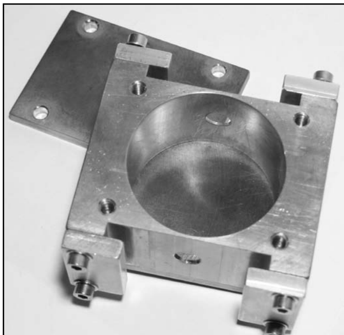
Figure 5 — Here is the cylindrical copper cavity for TE_{011} mode.
