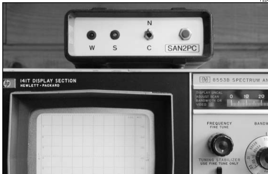
Figure 5 — The SAN2PC is a small package that easily sits on top of the HP141T spectrum analyzer.
