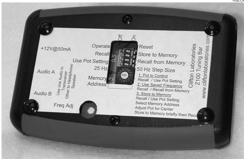
Figure 6 — To allow the use of a low profile enclosure, the operating controls are mounted to the bottom of the circuit board and access holes are cut in the bottom of the enclosure.
