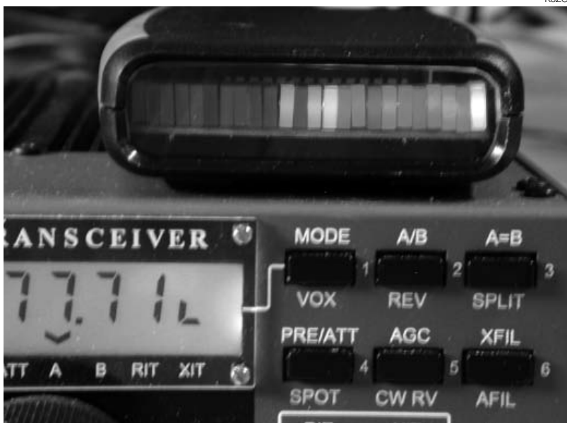
Figure 1 — The Z100 tuning aid sits atop the author’s Elecraft K2 transceiver.
