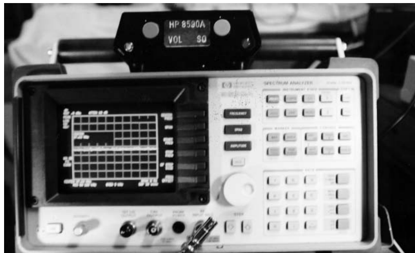
This photo shows the squelch amplifier connected to an HP 8590A spectrum analyzer, ready for operation.
