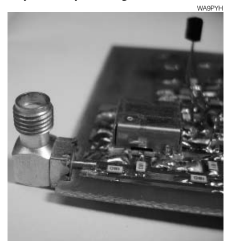
Figure 8 — The SMA output connector solders to the edge of the circuit board.
