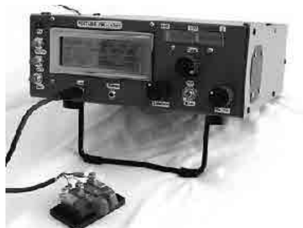
Figure 3 — We built this portable PSK unit around 2000. It was too complex and expensive, with separate boards for DSP and control processing. It did include a novel CW user interface.
