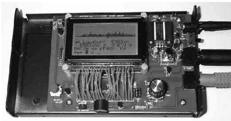
Figure 9 — This photo shows the NUE-PSK assembly. A 4 × 5 inch circuit board fits neatly into the enclosure, holding all components. (Individual wires are shown connecting the display in this prototype unit.) The battery "door" in the back of the case is visible along the left edge of the photo. Two 9 V batteries fit into the space between the circuit board and the case.
