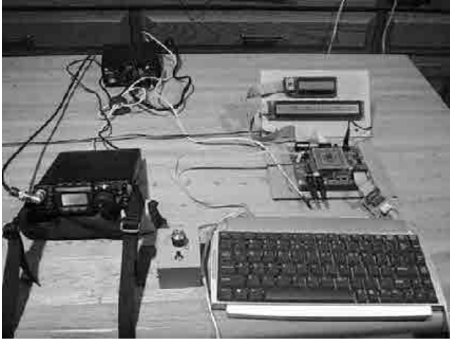
Figure 10 — NUE-PSK Prototype System. Clockwise from upper right: NUE-PSK displays and prototype hardware, standard PS2 keyboard, FT-817 transceiver, and power supply.
