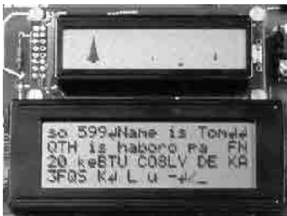
Figure 5 — The two-LCD Prototype used a graphic LCD for the spectrum display (top) and a character LCD for receive and transmit text characters (bottom).
