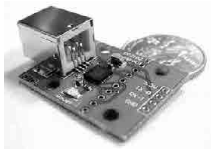
Figure 13 — A USB-to-TTL interface adapter from SparkFun will allow your computer USB port to connect to the modem for programming updates to the software.
