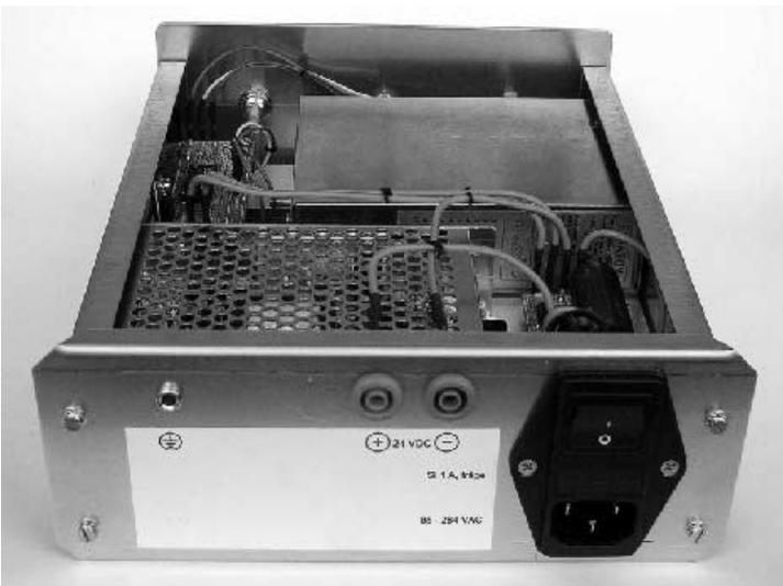
Photo C — This view shows the inside of DJ7GP’s rubidium oscillator from the rear panel.
