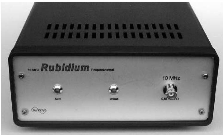
Photo A — DJ7GP built this version of John Raydo’s rubidium atomic frequency standard.
