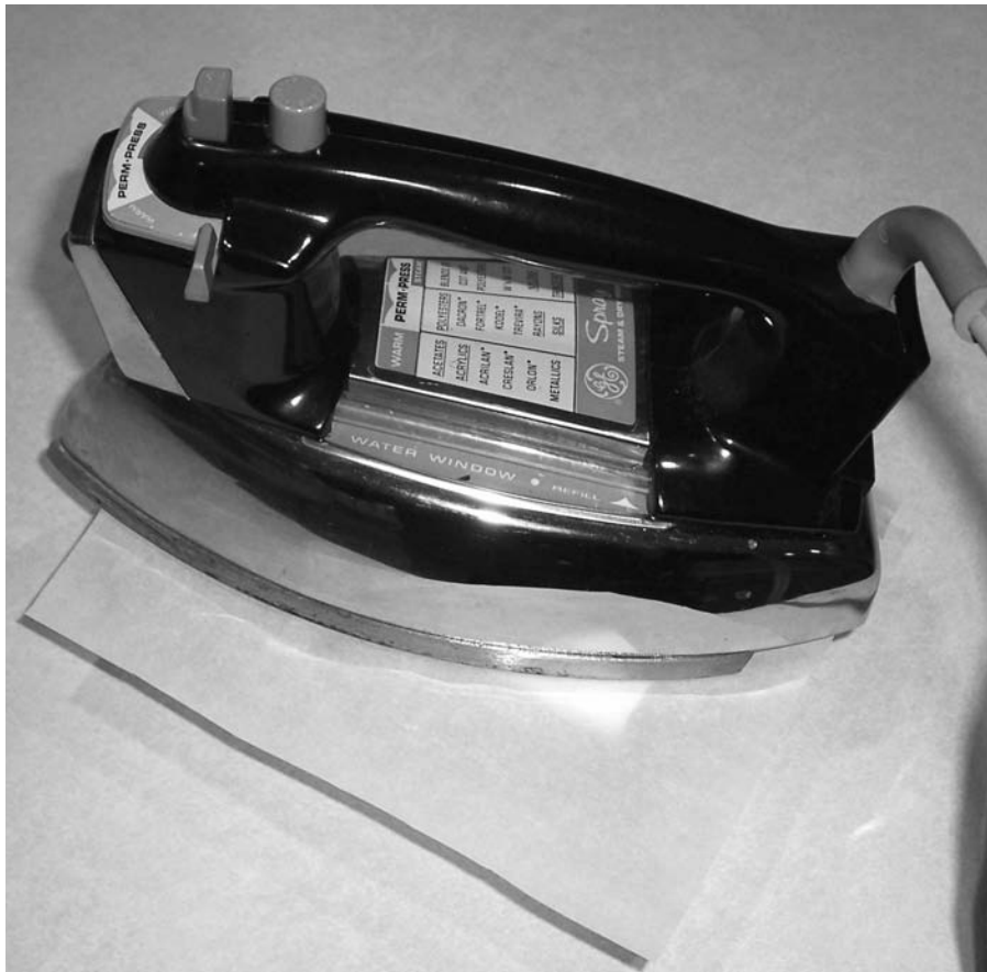
Figure 4 — The Press-n-Peel circuit pattern and parchment paper are placed on top of the material stack shown in Figure 3. Then the iron is used to heat the Press-n-Peel material to transfer the etch resist to the circuit board material.
