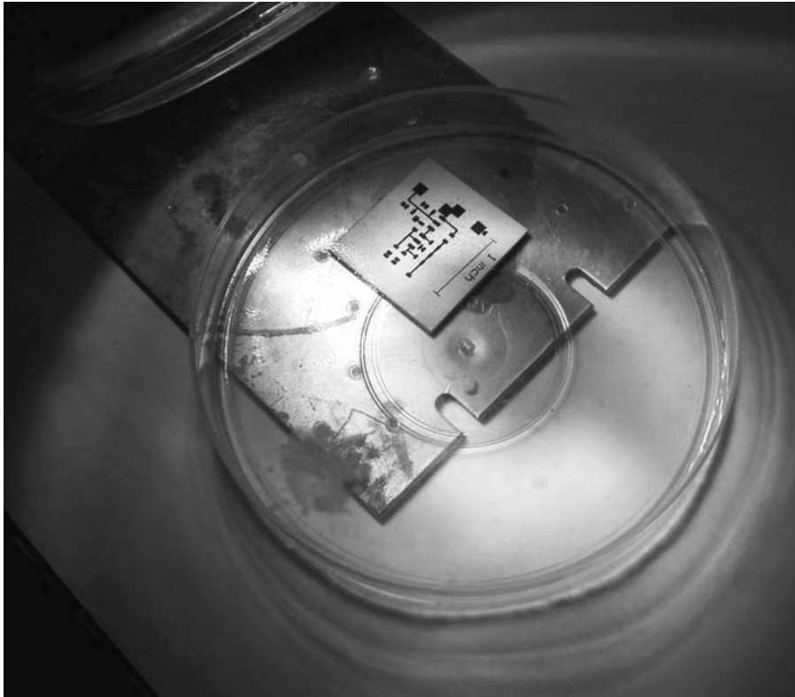
Figure 6 — The circuit board with resist is placed in a small plastic tray under the heat lamp.
