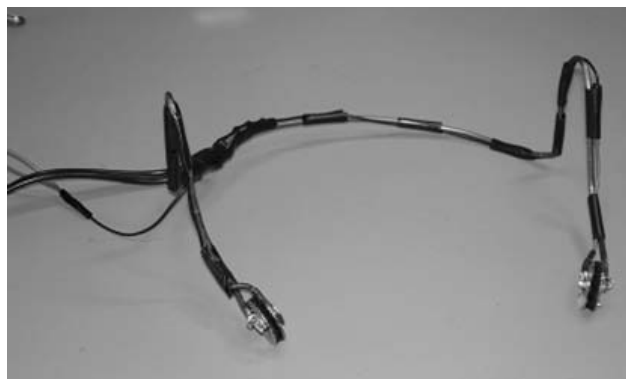
Figure E — Here, the electrodes are mounted on the ends of the wire-band.
