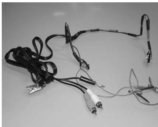
Figure F — Here is a photo of the completed wire band electrode configuration.
