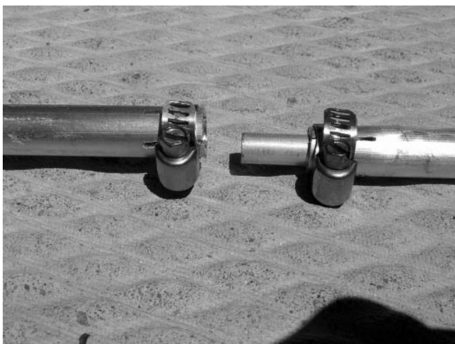
Figure 4 — This photo shows the 1.2 inch (30 mm) nipple cut from a piece of 1/4 inch aluminum tubing, which will be used to join the two sections of the driven element. Each side of the driven element tubing has a lengthwise slit in the tubing, so the hose clamps can compress the tubing and secure it to the nipple.
