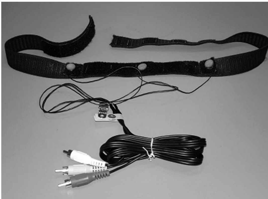
Figure B — This is a photo of an EMG headband electrode configuration.
