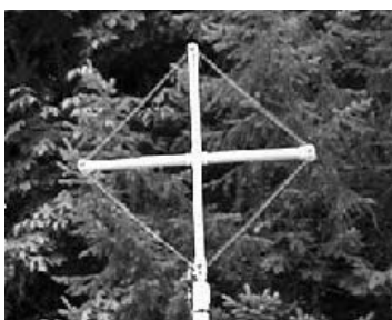
Figure 7 — This photo shows the loop receiving antenna.
