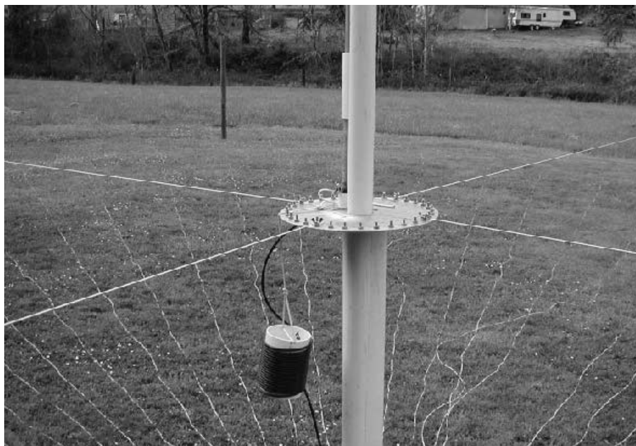
Figure 6 — The base plate is in position for elevated radials.
