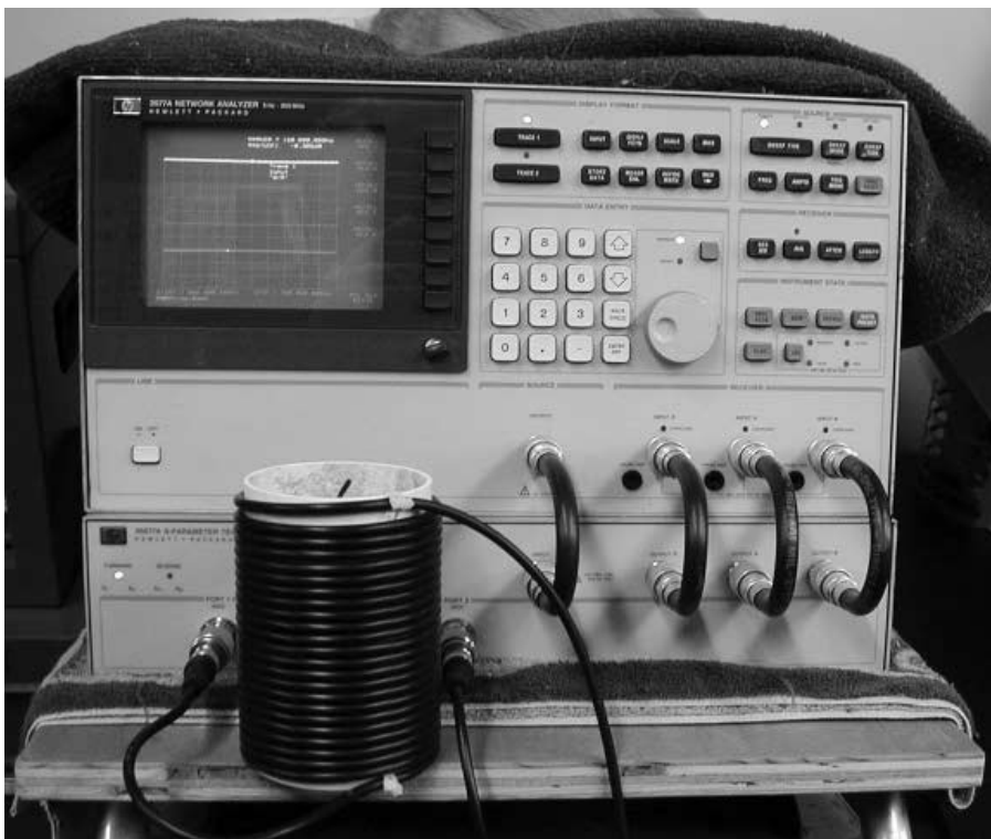
Figure 9 — HP3577A with an HP35677A S-parameter test box.
