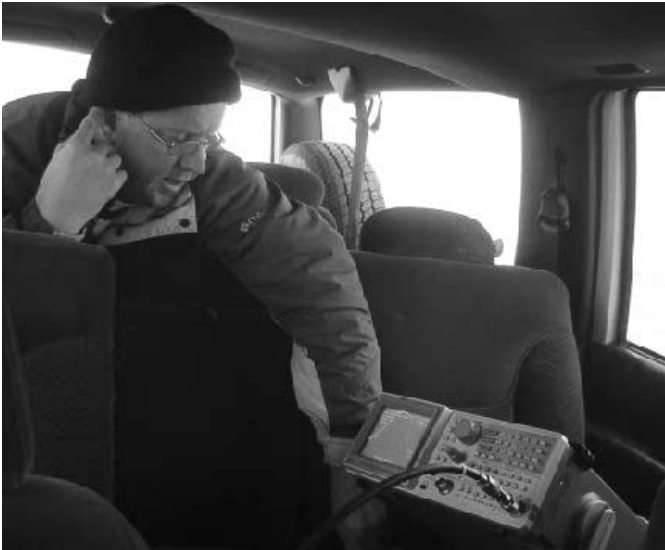
Todd Romriell reading the signal strength on the spectrum analyzer.
