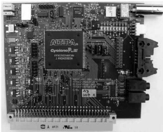
Photo 1 — This is the last of three Mercury prototypes. The TAPR production units will be identical to this hand-built prototype. The voltage regulators are along the left side. The 122.88 MHz low phase-noise oscillator is the large silver can in the upper left corner. The RF front-end circuitry is in the upper right corner; the RF signal flows from the BNC input on the right to the LT2208 ADC (square chip in the middle) where it is digitized and fed to the Altera EP3C25 Cyclone 3 FPGA (large chip in the middle). On the right edge, from bottom to top are headphone and line outputs; SPI interface to the Alex Preselector; and forward and reverse power signals to the analog converter on the Penelope transmitter. The 96-pin DIN connector along the bottom plugs into the Atlas backplane.
