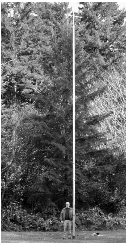
Figure 8 — Here is the receiving antenna atop a 40 foot mast. N7MQ assisting!
