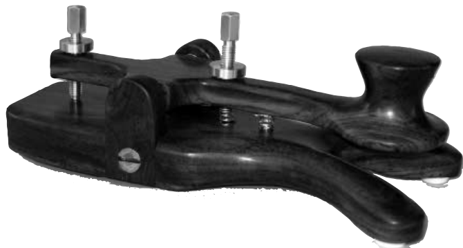
Morse keys are an old favorite of radio craftsmen. This one is made from a block of cocobolo and features custom-made hardware, silver contacts, and sealed ball bearings. The knob is carved asymmetrically to fit the owner's hand.
