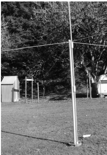
Figure 4 — This photo shows a typical test antenna and center post support.
