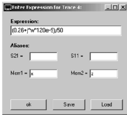
Figure 9 — VNWA software input mask showing the impedance formula of the lossy 120 nH inductor normalized to 50 Ω used in the simulation trace 4 of Figure 8.
