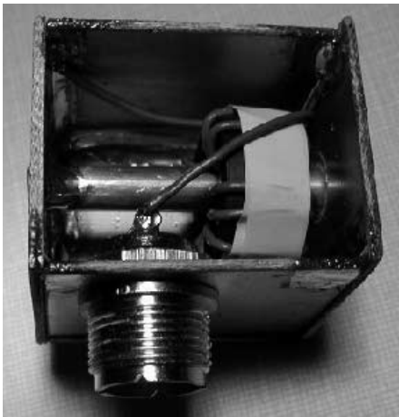
Figure 11 — This photo shows a typical shielded current transformer.
