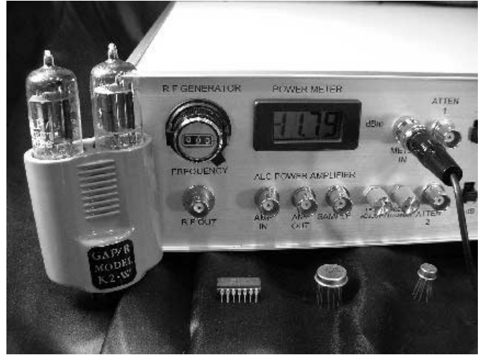
A K2-W operational amplifier and some more modern op amps are shown along with Gary Steinbaugh's homebrew spectrum analyzer.
