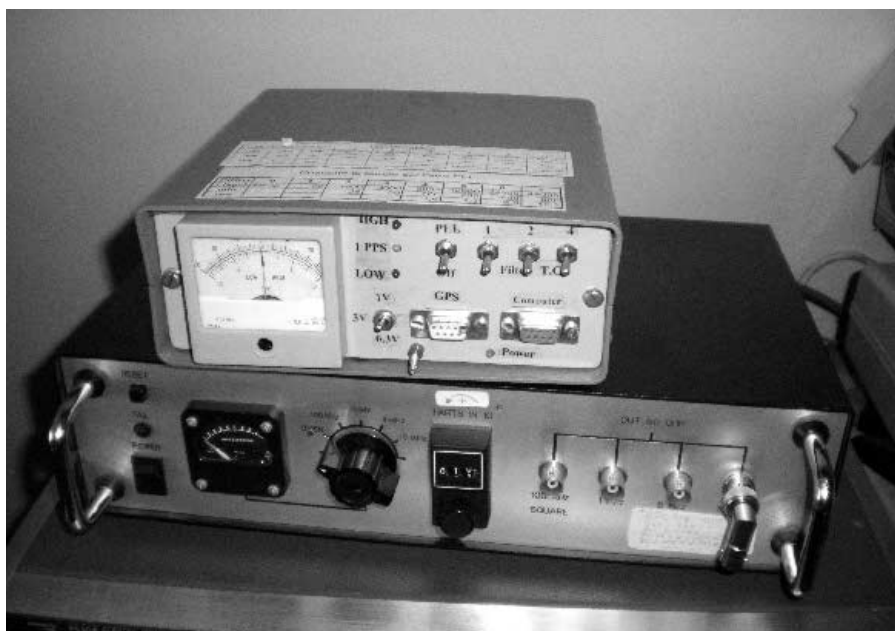
Photo 4 — Andrea Daretti, IZ2OUK, built the GPS-Based Frequency Standard from the July 1998 issue of QST. The top box is the "disciplinizer," and the quartz crystal oscillator is under that.
