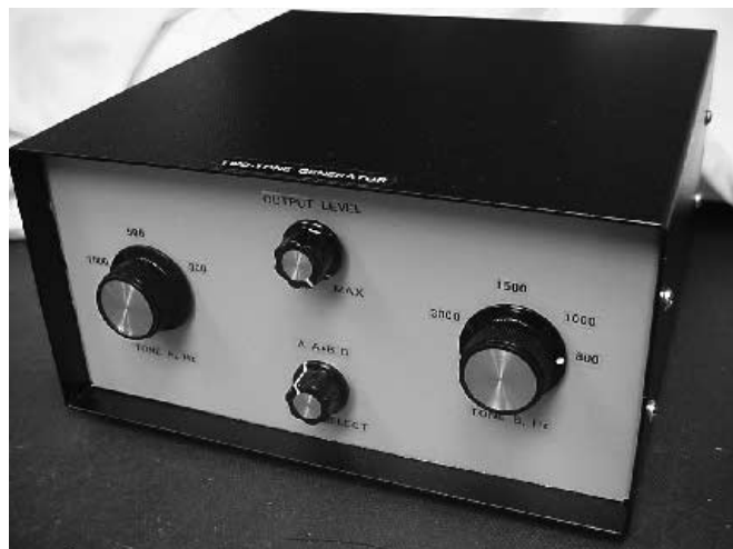
Figure 2 — Front panel view of the two-tone generator. Note the individual controls for Tones A and B.
