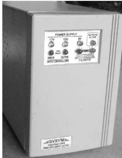
Photo 2 — This photo shows the front panel of Taso's GPS-derived frequency standard. He used two LEDs for the FLL status indication, instead of a single bicolor LED.
