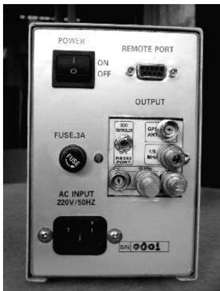
Photo 3 — Here is the back panel of Taso's project. Using 50 Ω terminations at the unused outputs proved beneficial.
