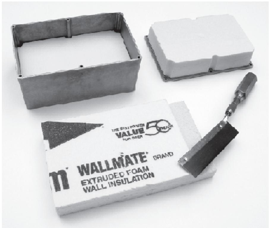
Figure 21 — To increase the crystal temperature to 75°C, the circuit board, crystal and heating element are sandwiched between layers of 1½ inch thick expanded polystyrene insulation, readily available at home improvement stores. This foam is easily cut with a fine-tooth razor saw, and with care it can be shaped and smoothed with sandpaper.
