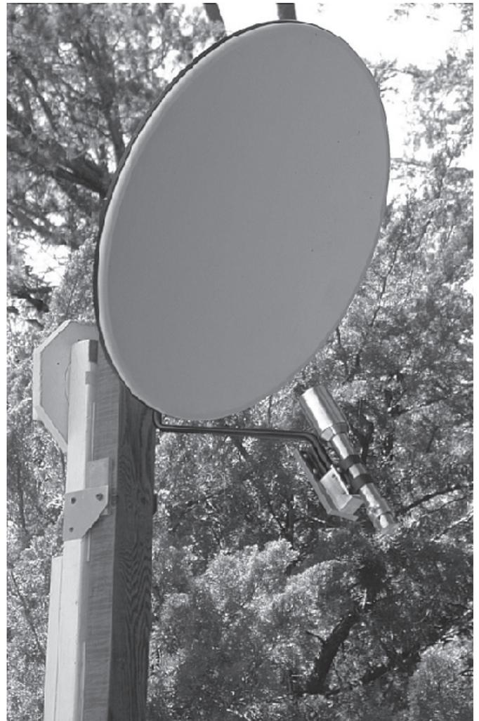
Figure 18 — A W6VSV 18 inch off center fed satellite TV parabolic dish, with a homemade 10.368 GHz dual mode feed horn is attached to the antenna test fixture.
