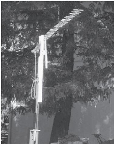
Figure 12 — A KLM 45 element 1296 MHz Yagi is attached to the antenna test fixture.
