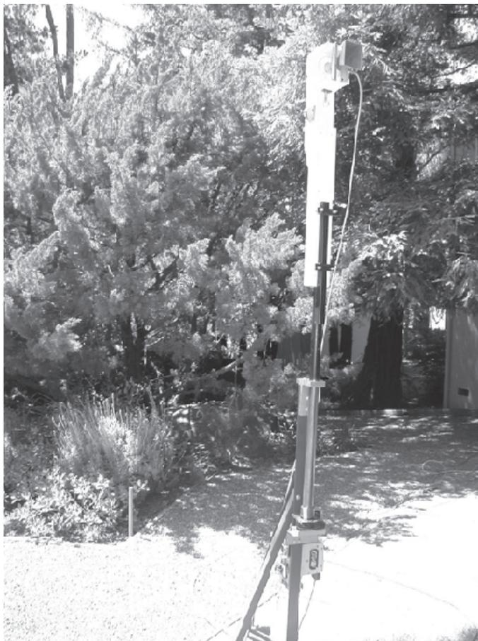
Figure 16 — A WWII X-band radar test horn is placed on the antenna test fixture.
