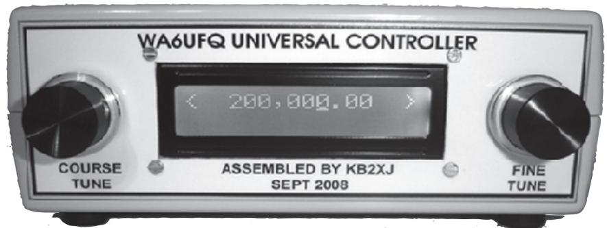
Figure 1 — This VFO controller was built by James Elledge, KB2XJ. Jim used a PacTec LH64-200 enclosure, and a white on blue LCD.
