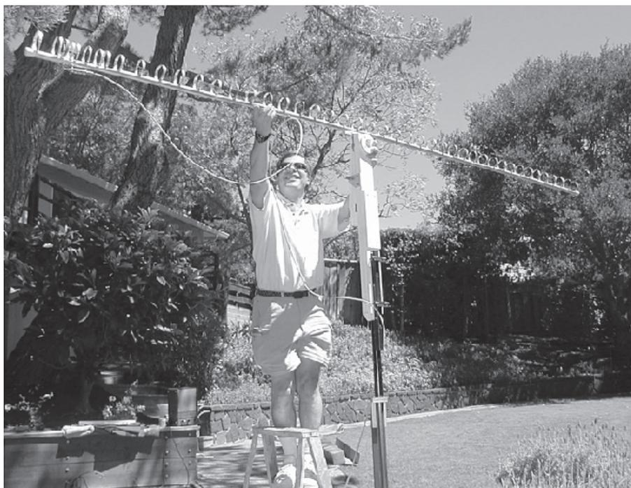
Figure 14 — A W6PQL 45 element 1296 MHz loop Yagi is prepared for testing.
