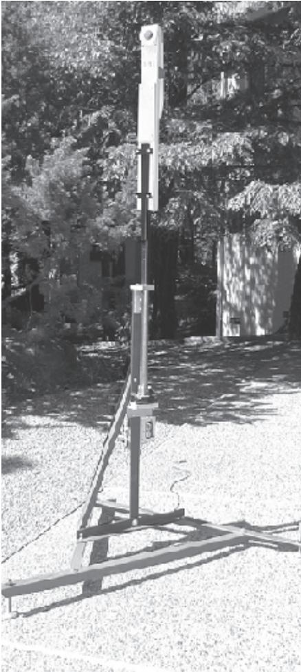
Figure 8 — Here is a close-up view of the 9 foot tall rotating antenna test stand. The base frame includes leveling screws to ensure that the antenna is level and plumb. The antenna is rotated by a stepper motor with a 50:1 gearbox. At the top is a structure that can tightly clamp on Yagi booms or many other types of arrays. The clamping arrangement permits easy polarization rotation when making both E and H plane plots.
