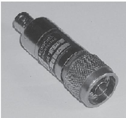
Figure 10 — This microwave crystal diode detector connects to the test antenna, and its 1000 Hz output signal is fed into the high gain, narrow bandwidth amplifier.
