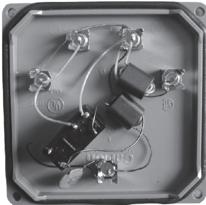
Figure 12 — End-fire directional control built into the cover of a "marine grade" plastic electrical box. Be sure to drill holes in the box to allow moisture out.
