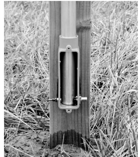
Figure 17 — A close-up view of a vertical element sitting inside bottom support enclosure.
