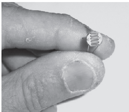
Figure 6 — Individual photo-resistor used in power meter. This is the largest resistor in the pack of five. Note the serpentine structure of the resistor.
