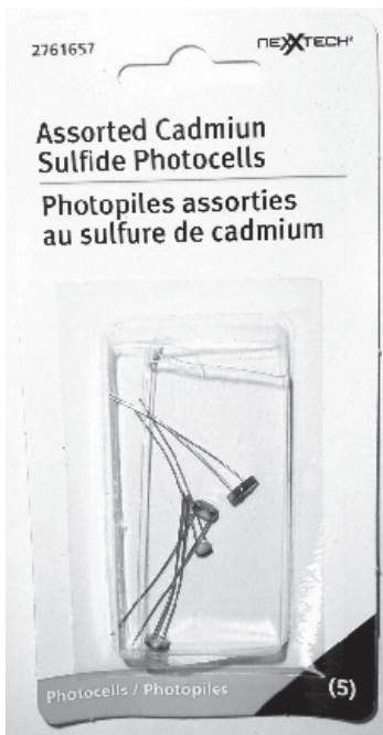
Figure 4 — Cadmium-sulfide photo-resistors available from RadioShack in a pack of five.
