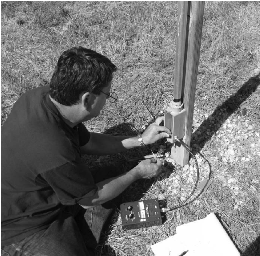
Figure 20 — W5ZN measuring the self-resonance of the vertical elements.
