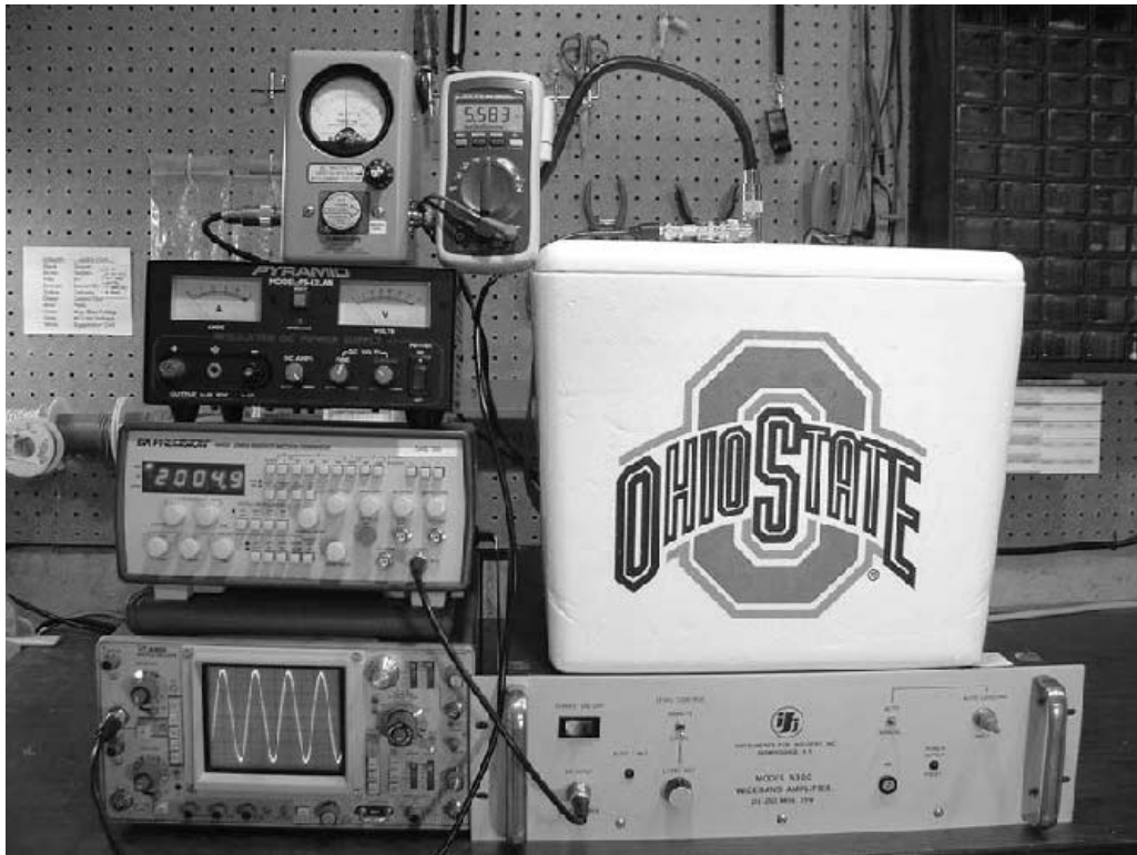
Figure 8 — This photo shows the equipment set-up used to verify the wattmeter operation and accuracy.
