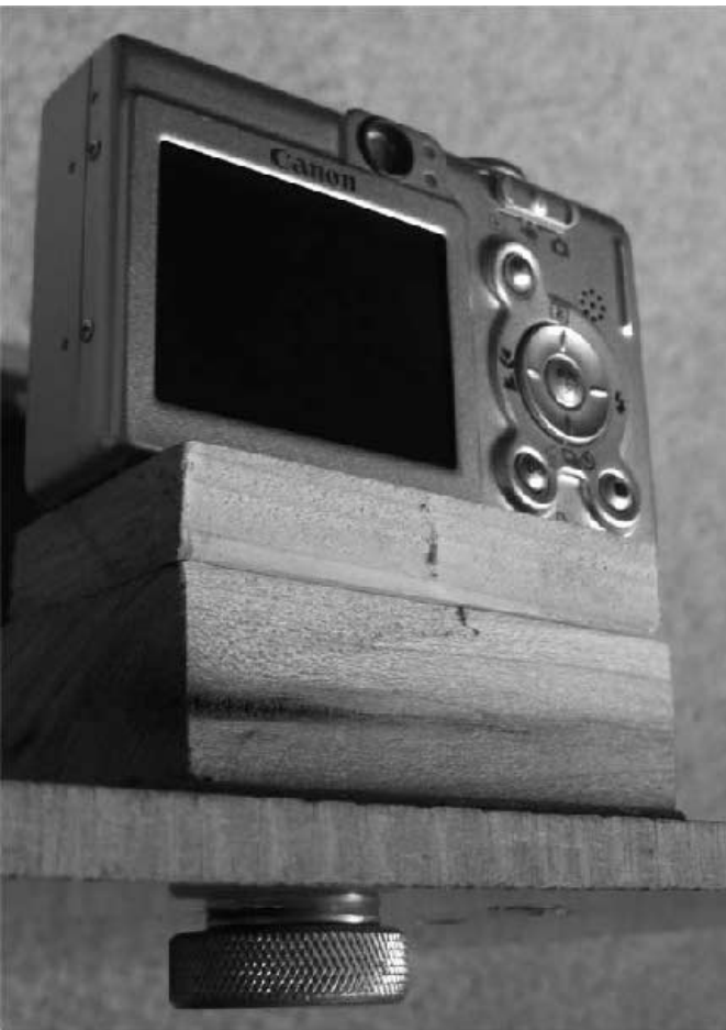
Figure 7 — This photo shows the spacer boards used to shim the camera to the proper height so the lens will be centered on the oscilloscope display.
