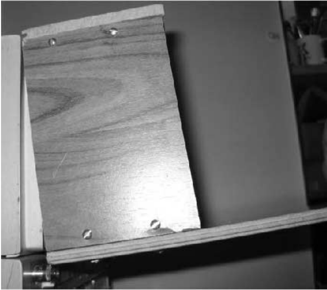
Figure 6 — The screw points in the top board fit into the V groove of the oscilloscope frame, and the mounting system hinges down into position.
