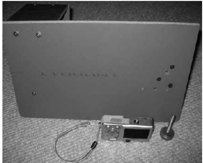
Figure 9 — Viewed from the bottom of the camera mounting system, you can see that there are several holes to accommodate the “swivel pad clamp” screw for attaching various cameras for proper positioning of the camera lens.
