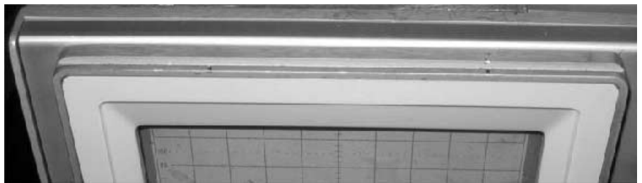
Figure 4 — The top edge of the frame around this Tektronix oscilloscope has a V groove designed to hold a camera mount. The author drove two wood screws through the top of his camera mount box so the points of the screws protrude just enough to engage in this groove.
