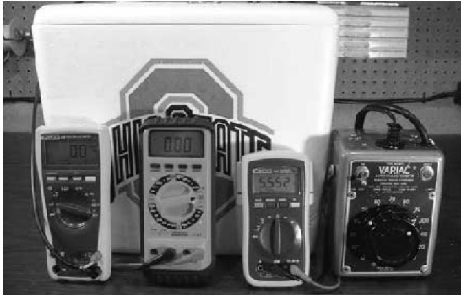
Figure 4 — This photo shows the completed calorimeter along with the various meters and variable transformer that the author used to calibrate the system.
