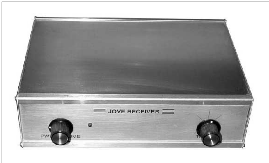
Figure 2 — The Jove RJ1.1 direct conversion receiver is simplicity itself with only two controls – a POWER SWITCH/VOLUME CONTROL and a TUNING knob. Low level audio from the receiver is sent to a computer sound card and also may drive an amplified speaker. The receiver uses a J310 grounded gate RF amplifier followed by the traditional NE602 mixer/oscillator and high gain audio amplifiers. A varicap tunes the receiver over a 400 kHz range centered on 20.1 MHz.
