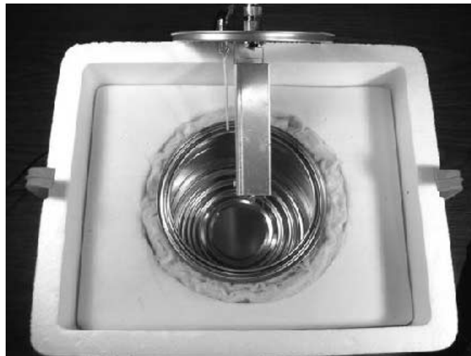
Figure 3 — Here is the paint can and insulation inside the foam cooler. The can is filled with transformer oil before the resistor and thermistor assembly is lowered into the can and the lid closed.
