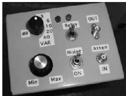
Photo 1 — Ron Skelton, W6WO, built this "Controlled Noise Source," with a calibrated noise source and switched PIN diode attenuator.
