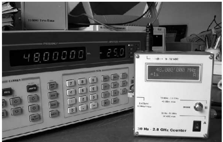
The frequency counter in this project is connected to a commercial RF generator.
