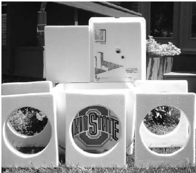
Figure 2 — Pieces of foam insulation were cut to fit snugly around the dummy load paint can and fill the inside of a Styrofoam cooler. Note that the logo on the cooler can be one of your choice.
