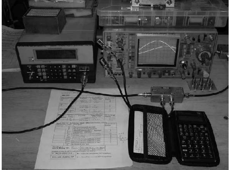
Figure 18 — Impedance tests being performed with careful logging and storage of measurements.
