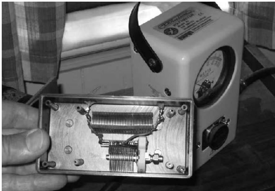
One of the original traps used with this antenna. It is comprised of a 10  $\mu H$  B&W miniductor coil and a Johnson 158-5-23 air variable capacitor set to 33.5 pF.
