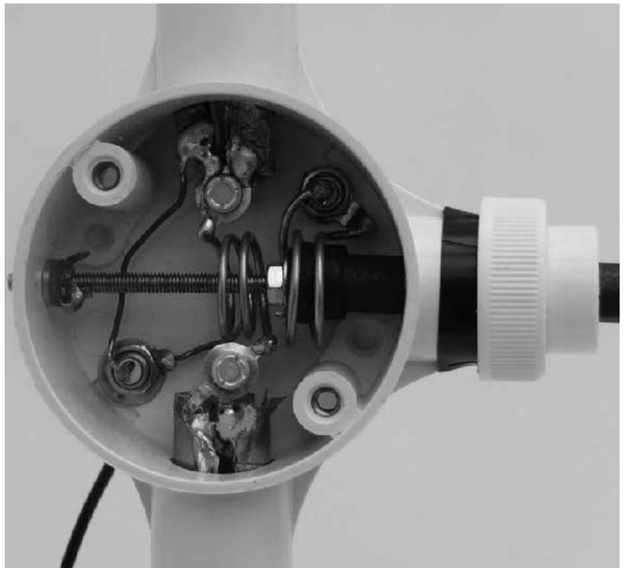
Figure 3 — PVC T box showing the adjustable ferrite rod and the coil in series with loop elements. The coil on right is an inductive coupling
