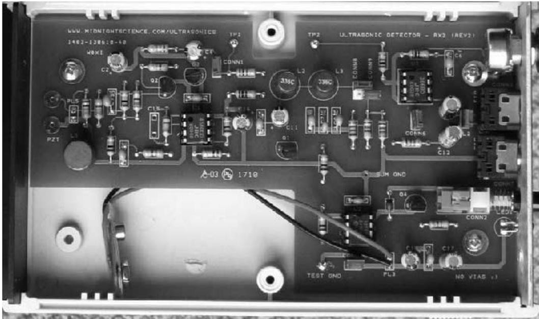
Figure 7 — The AGC circuit is incorporated into the circuit board for the Ultra-RX2 ultrasonic receiver. The AGC circuit is in the top left corner of the circuit board. Note that the component designators on the board may not match the designators on the schematic of Figure 6.
