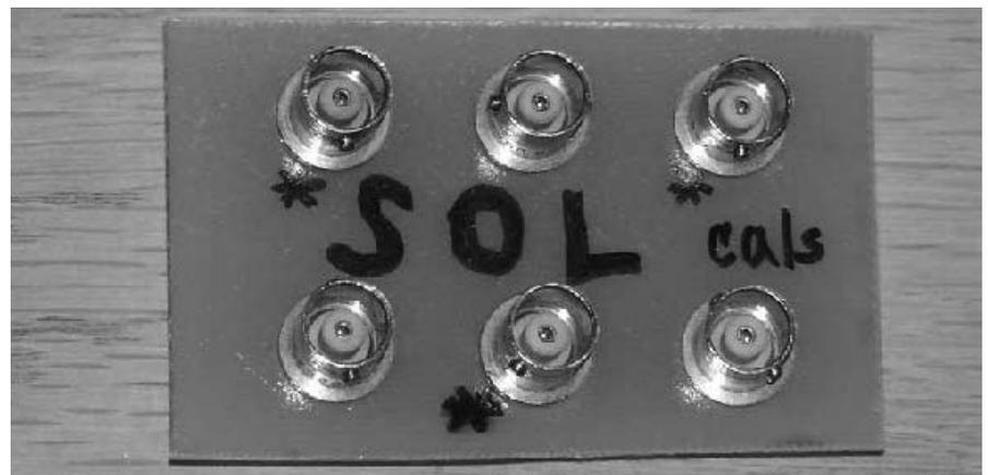
Figure 7 — The breadboarded SOL calibration "standards." I tried different ways of making the loads, so there are extras just for the sake of experiment.
