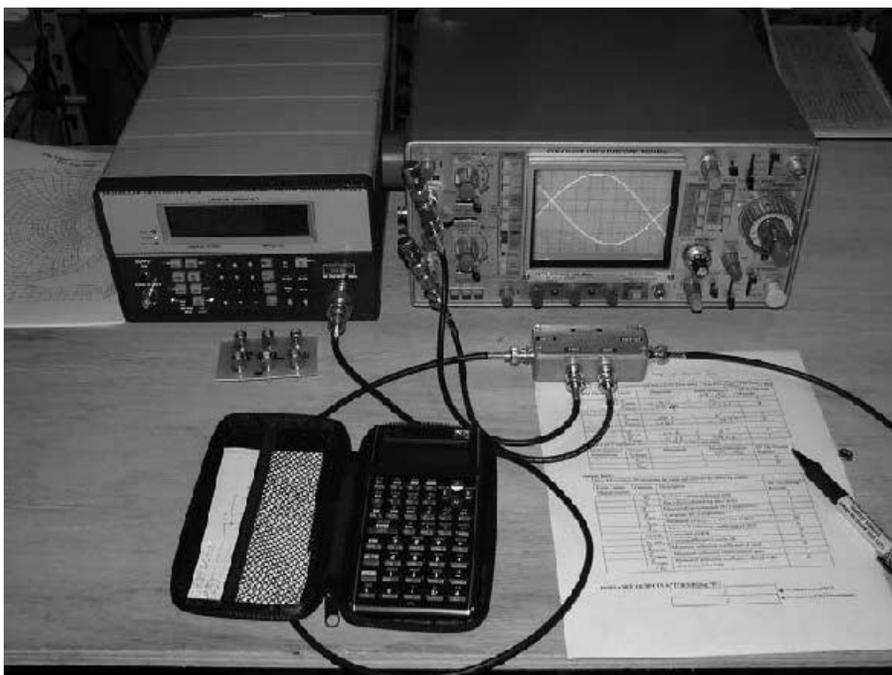
**Figure 11** — The bench-top system. This is all there is to it: a coupler, a signal generator, an oscilloscope, a DUT test cable, a checklist, the SOLs, and a programmable calculator.
