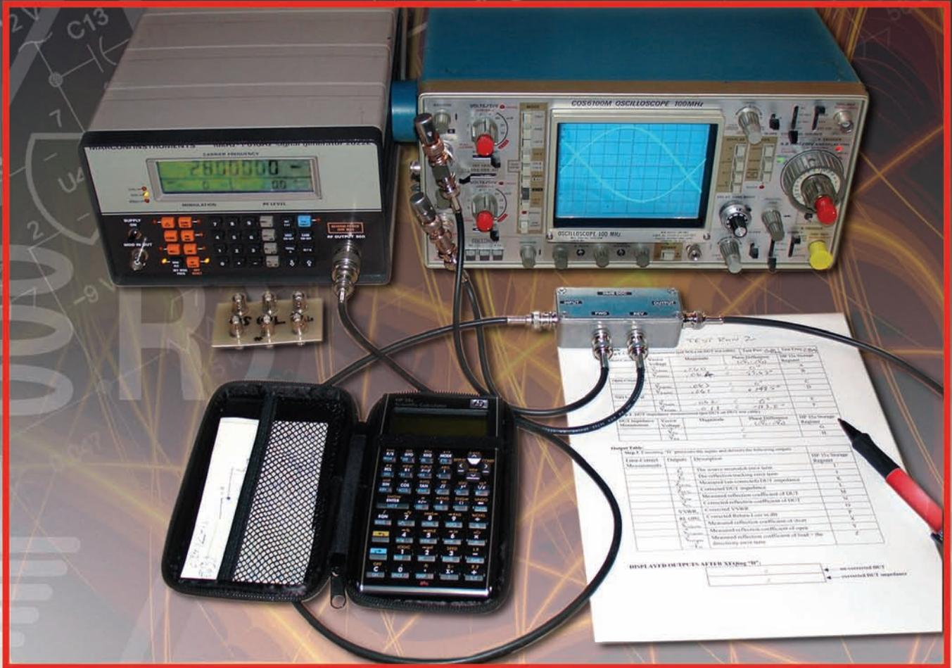
**KG2MG** shows you how to make complex impedance measurements with a bidirectional coupler and an HP 35s calculator.
