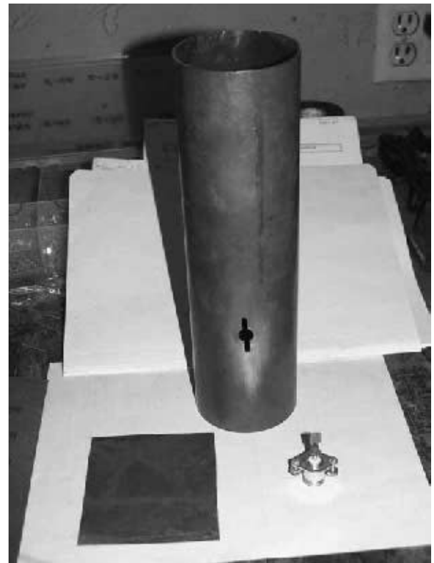
Figure 9 — Materials ready for assembly. The cut cylinder, copper plate, for closing the end of the pipe, and the probe assembly.
