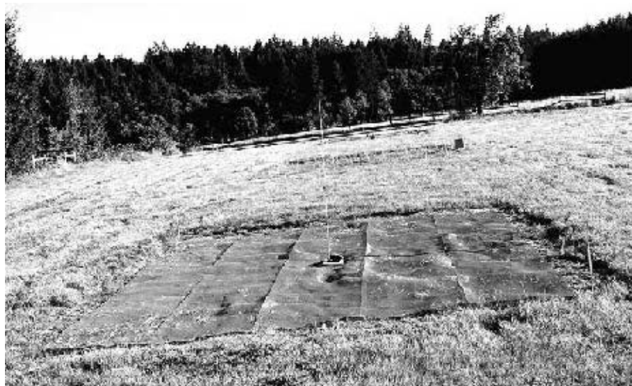
Figure 1 – Our mesh ground screen in foreground, buried radials at center and elevated radials in the distance
