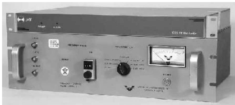
Figure 1 – The complete 10 MHz Frequency Standard distribution system. The 10 MHz output from the modified Vectron FS321A-1 frequency standard is sent to as many as 12 loads by the Precision Time and Frequency, Inc. Model 1203C distribution amplifier.
