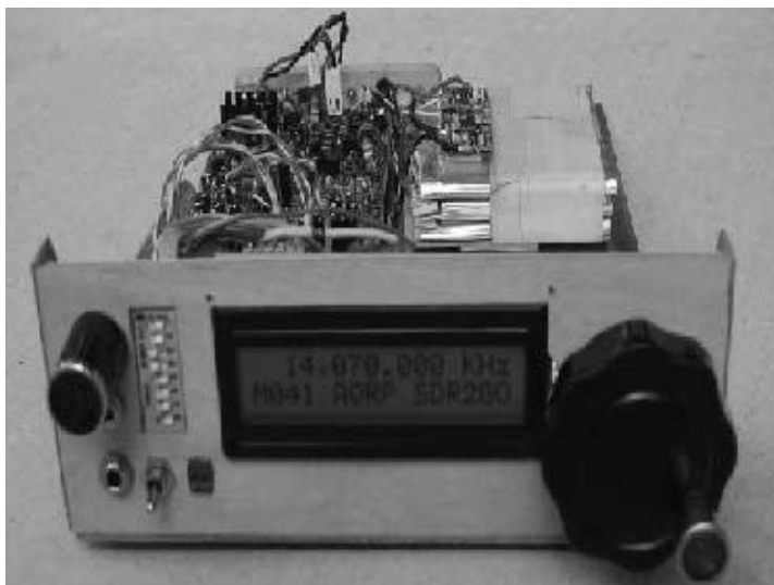
Figure 6 – Front panel of the author's transceiver
