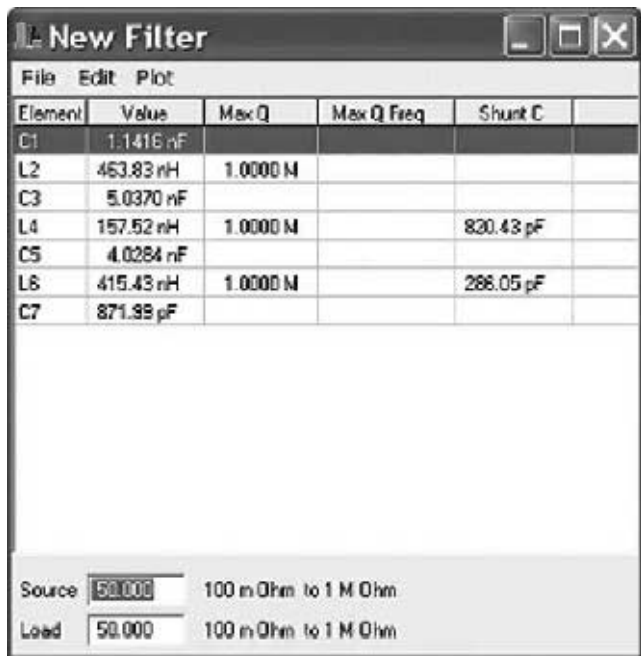
Figure 14 — The element values can be viewed and modified from the element list window.
