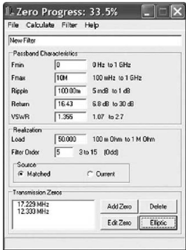
Figure 10 — The application can calculate and insert zeros required for an elliptic filter.
