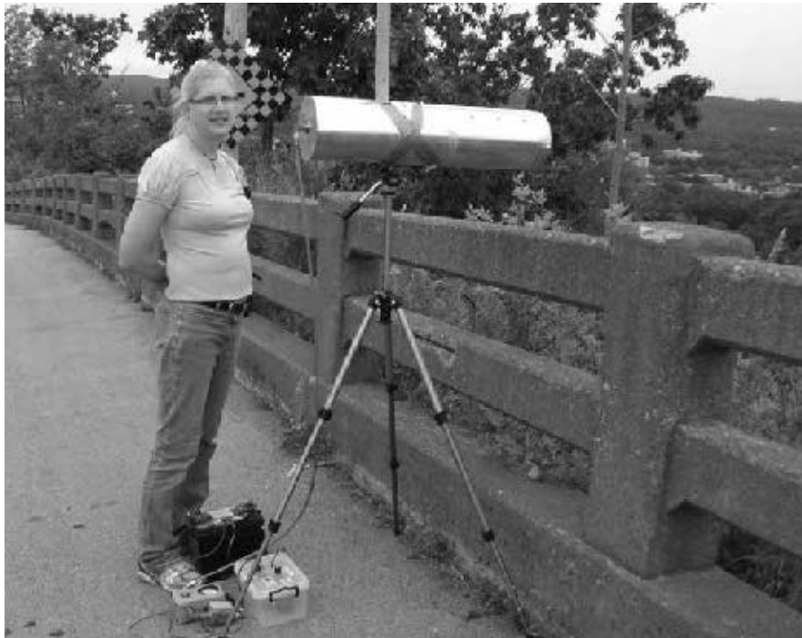
Figure 9 — Sherry Goeller, VE3DCU, operating the transmitting momentum station on the 1500 m link. Note that the coaxial cable is connected to the rear of the waveguide.
