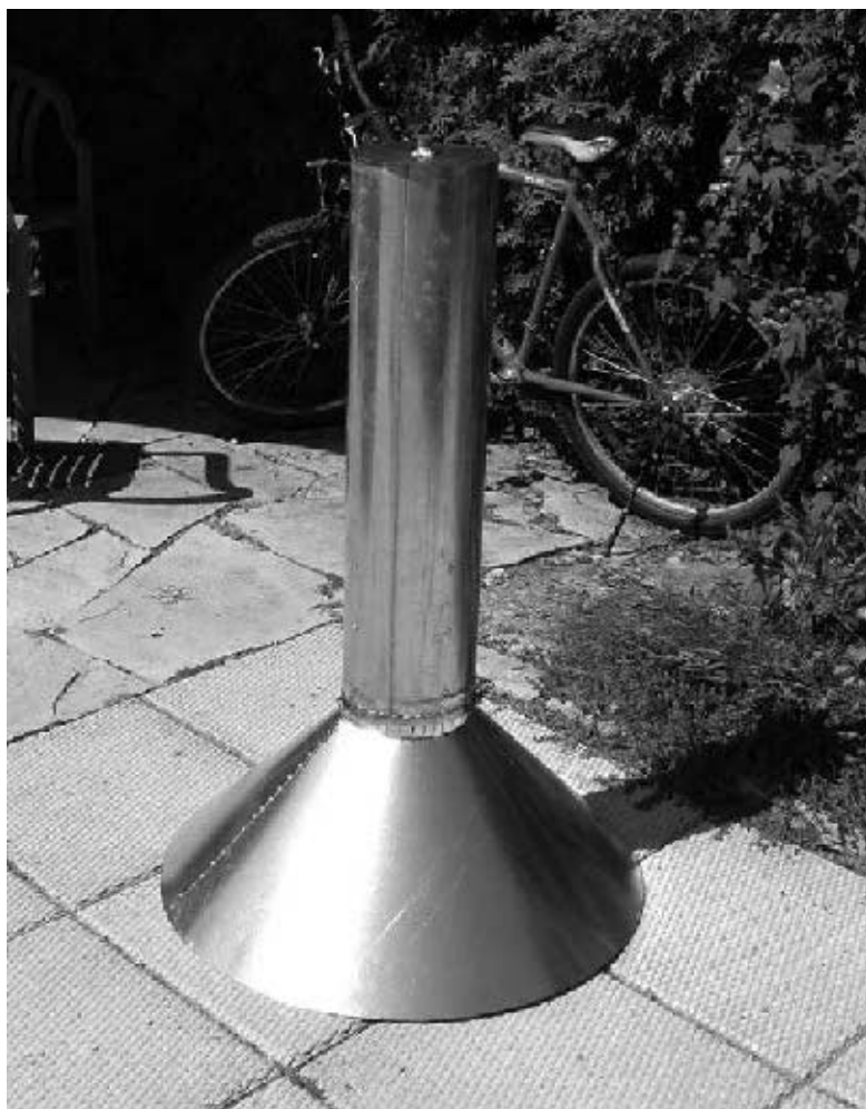
Figure 8 — The 20 dBi gain conical horn built for the receiving detector is shown here.
