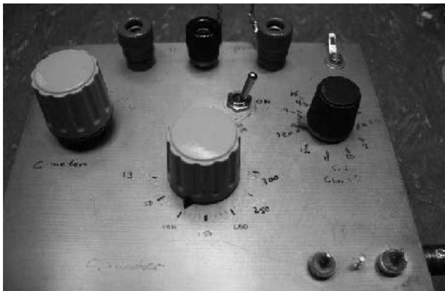
Figure 5 — Front view of the prototype equipment. It includes C-meter, gray knob and red banana terminal on the left that is not included in this presentation. The coil terminals are black and red on the right.
