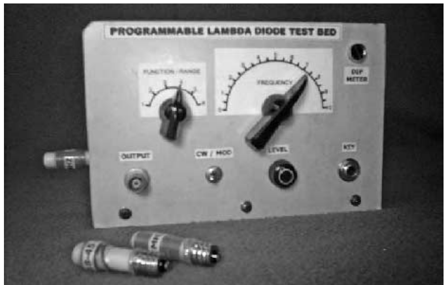
The author's test bed used to experiment with a variety of lambda diode applications.
