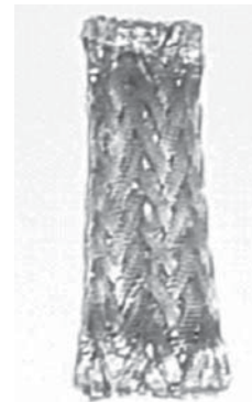
Figure 10 — Here is a length of coaxial cable braid, pre-tinned so it is ready to be soldered to the conducting plates.
