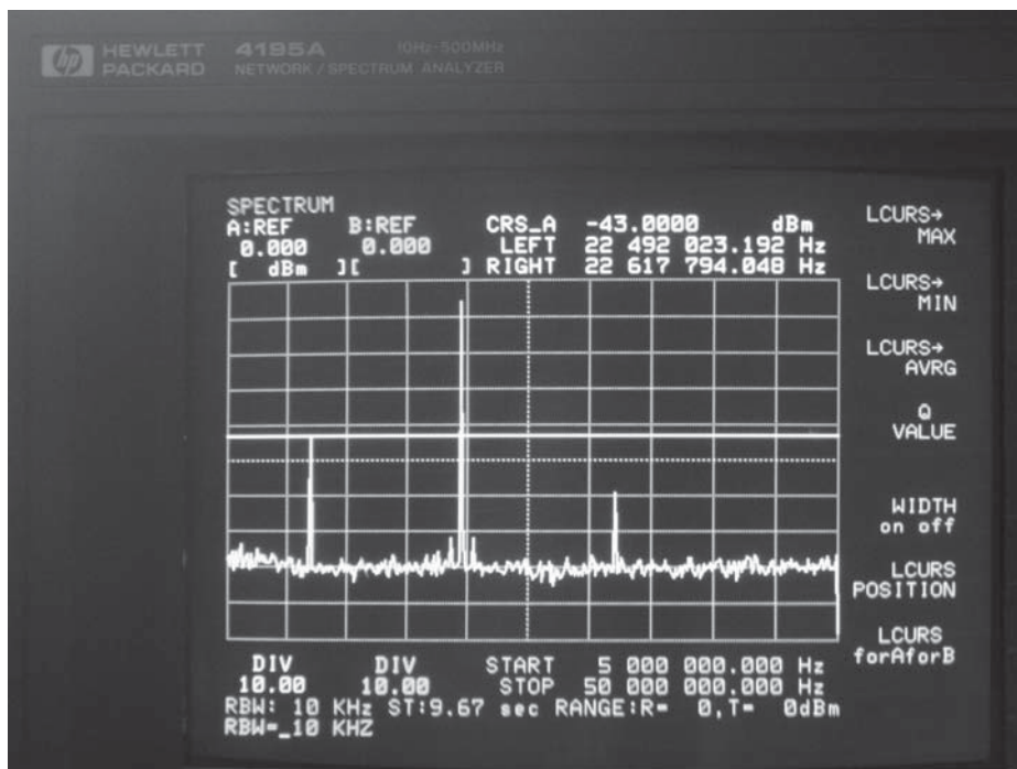
Figure 6 — This spectrum analyzer display shows the spectrum of the 22.625 MHz signal from the frequency doubler circuit. This signal is used as the synthesizer reference signal for my Yaesu FT-587D transceiver.
