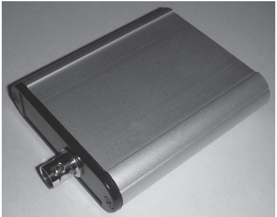
Figure 6 — The Simple SDR receiver board will fit inside a Hammond Manufacturing model 1455B802 enclosure if a chassis-mount BNC connector is used instead of the on-board connector.
