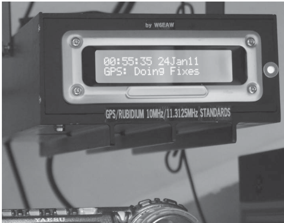
Photo 1 — Here is a front view of the main enclosure, with the LCD Monitor for the GPS unit.
