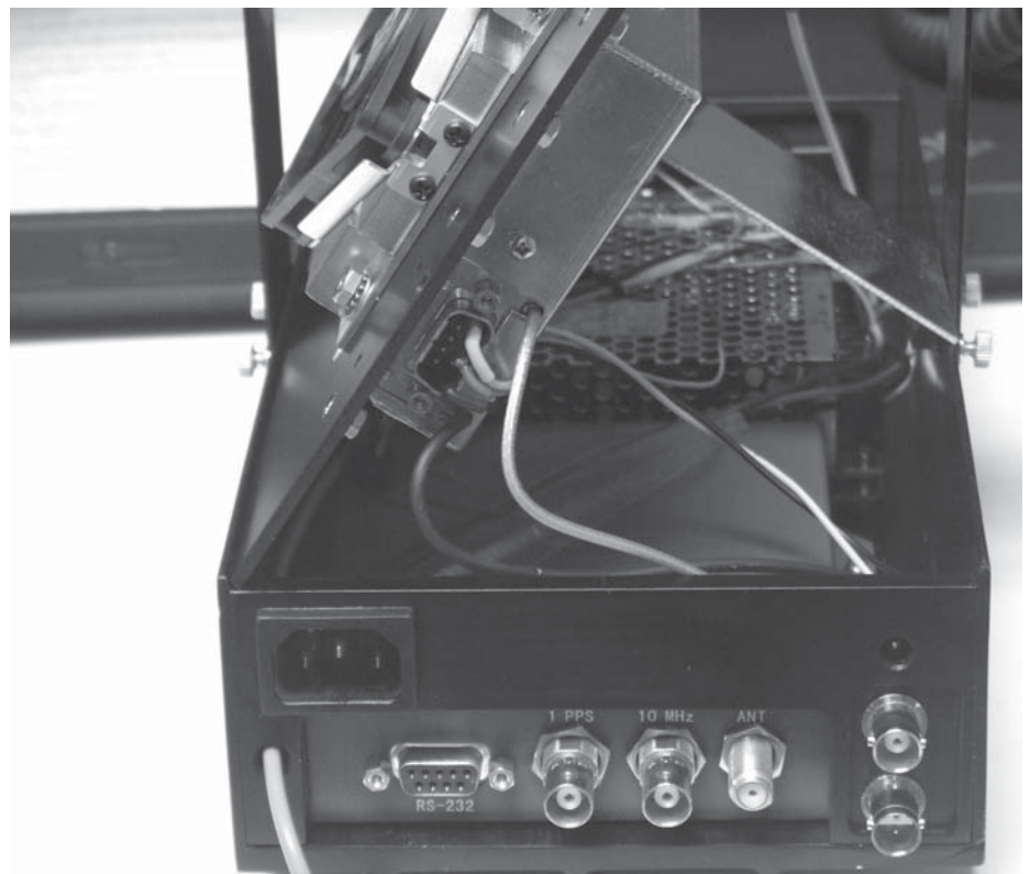
Photo D — This photo is an end view of the main enclosure that holds the Thunderbolt GPS, Thunderbolt Power Supply, and Rubidium Oscillator. On the top cover opposite the Rubidium Oscillator is the heat sink and fan.
