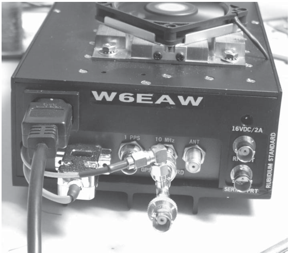
Photo H — This is the back panel of the main enclosure. Notice the T adapter on the 10 MHz output from the Thunderbolt GPS unit. The coax on the top of the T goes back inside the enclosure, to the PLL circuit board. The straight end of the T accepts the coax that carries the 10 MHz reference signal to the “special attenuator” (see Figure 1) and then to the ICOM IC-7800 transceiver.
