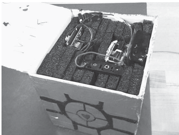
Figure 14 — Balloonsat payloads were constructed by folding \frac{3}{8} inch thick foam-core board into a cube shape approximately 6 inches on a side. The cubes were covered with adhesive-backed aluminum tape and the interior filled with automotive-type foam to provide insulation from both thermal and mechanical shocks.
