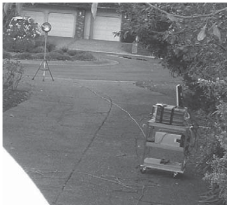
In this photo, a pair of 144 MHz Launchers are being measured with 100 feet of no. 24 magnet wire conductor in the driveway at N6GN. The vector network analyzer used for the measurement can be seen to the right, between the two ends.
