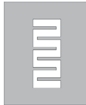
Figure 4 — The interdigital filter DGS element showing only the bottom copper pattern.
