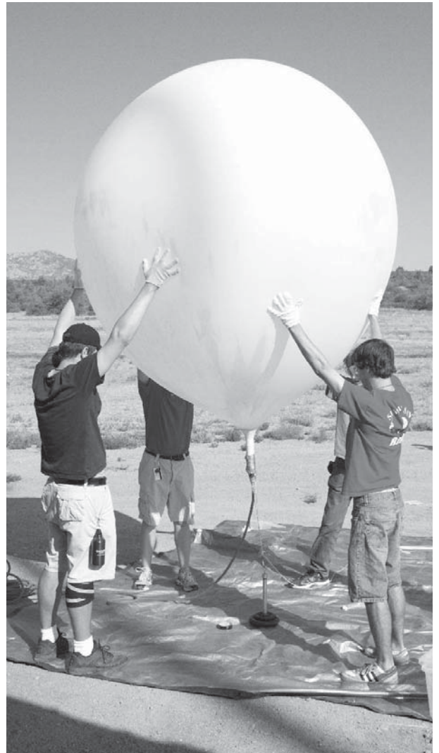
Figure 17 — Four students act as “handlers” to stabilize the balloon during inflation. The balloon is tethered to 15 pounds of weights to give an approximate indication of the amount of lift the balloon provides.
