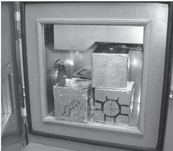
Figure 16 — Balloonsat payloads were placed in a thermal chamber, which was cooled to approximately -40^{\circ}\text{C} to simulate the temperatures encountered during flight through the troposphere.
