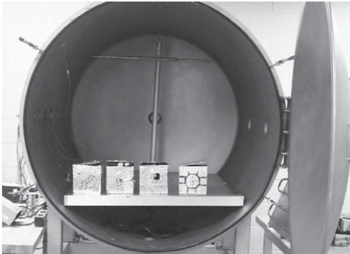
Figure 15 — Balloonsat payloads were placed in a vacuum chamber from which the air was evacuated to simulate a flight to 100,000 feet.
