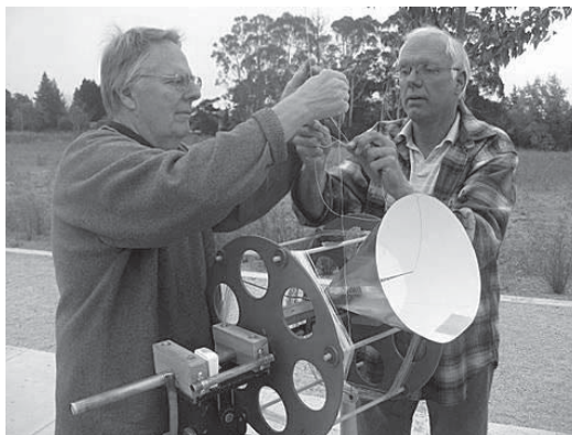
Completed 400 MHz launcher mounted on a "holder." The no. 24 SWTL conductor extends from the center of the horn and can be seen as a faint line in this photograph.
