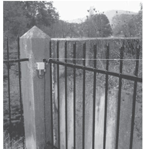
Figure 16 — Beverage antennas are always mounted close to the ground. Here you can see one of the feed points of my antenna, which is installed along the fence of my garden.
