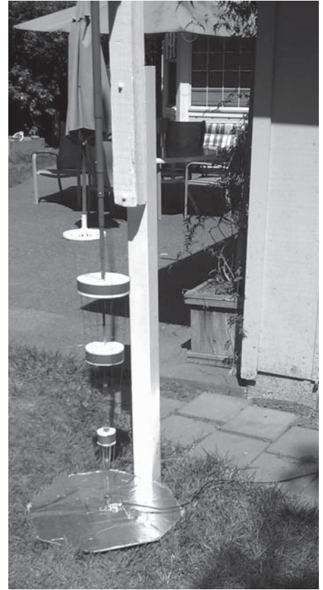
Photo 7 — The All-Band Antenna measurement setup is shown in these photographs. On the left it is being operated only as a simple vertical with good grounding. For the photograph on the right the SWTL launchers and VHF+ antenna are present. In addition to the hexagonal aluminum foil disk, which provides a good VHF ground, an 8 foot ground rod near the wooden post is also connected to the disk. This arrangement was left in place for all measurements even though the disk is not necessary when the launcher is in place.
