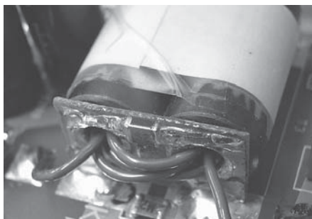
Figure 1 — Here you can see a 16 gauge, 4 turn winding in a binocular core.
