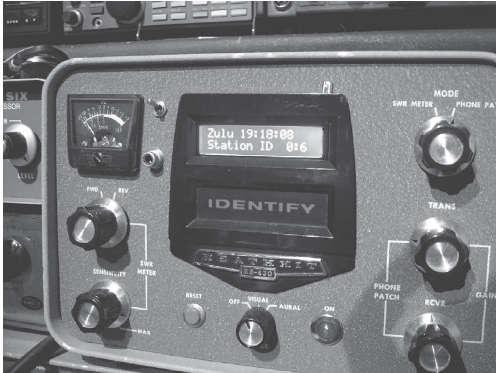
Here is the finished SB-630 showing the new ambient light sensor at the top right of the bezel. Also, the LCD is white on blue. Note that the RCA jack and toggle switch to the left of the bezel are for a modification to the phone patch for a different receiver input, which is not included in this Arduino project.
