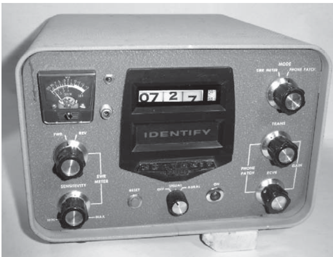
Original (circa 1960) SB-630 station console with a slight mod to switch audio from another radio into the phone patch.
