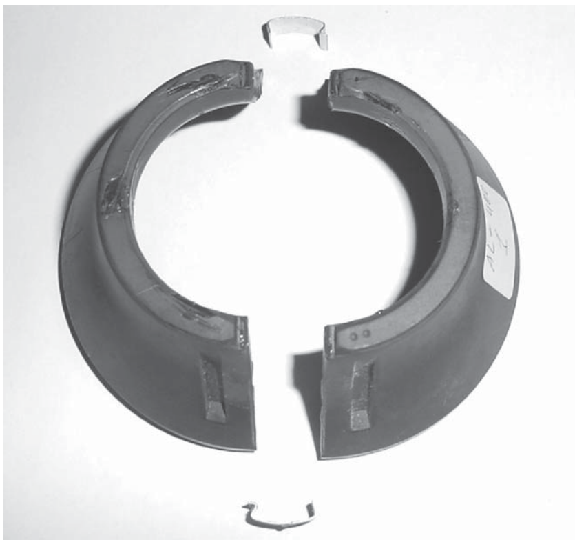
Figure 1 — A cathode ray tube yoke core. The steel clips hold the two halves together.
