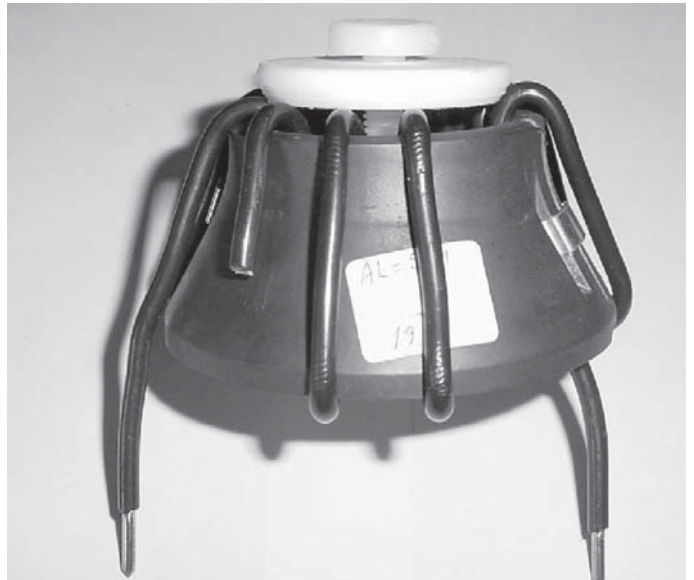
Figure 6 — A side view of the finished inductor showing the plastic mounting hardware.
