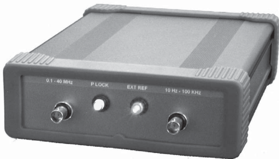
Figure 1 — The Direct Digital Synthesizer is packaged in extruded aluminum housing. Front panel BNC connectors are provided for the 10 Hz to 100 kHz and the 100 kHz to 40 MHz output. LED lamps indicate lock status of the reference PLL and the presence of an external 10 MHz reference input.
