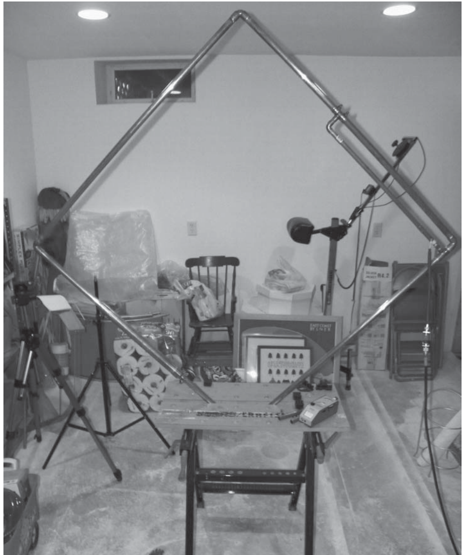
Figure 2 – The 42 × 42 inch loop under test in the author’s basement.
