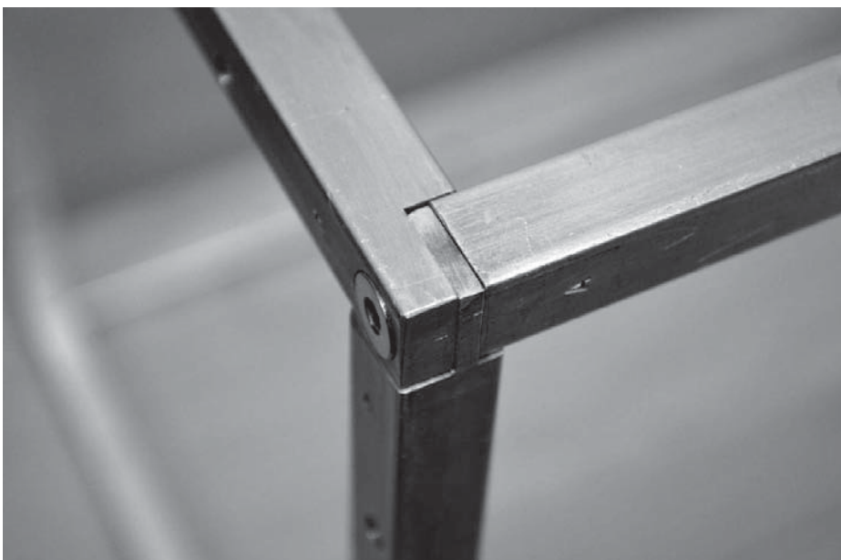
Figure 7 — The rectangular frame is constructed from ½ inch square aluminum stock. A single 10-32 flathead screw secures the three interlocking pieces that form each corner.
