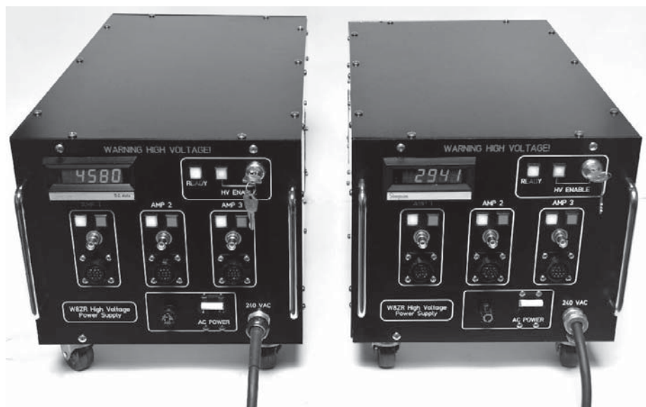
Figure 1 — The two high voltage power supplies are identical, except for different voltage ranges. Each rests on the floor behind an operating table and independently powers up to three legal-limit RF power amplifiers.
