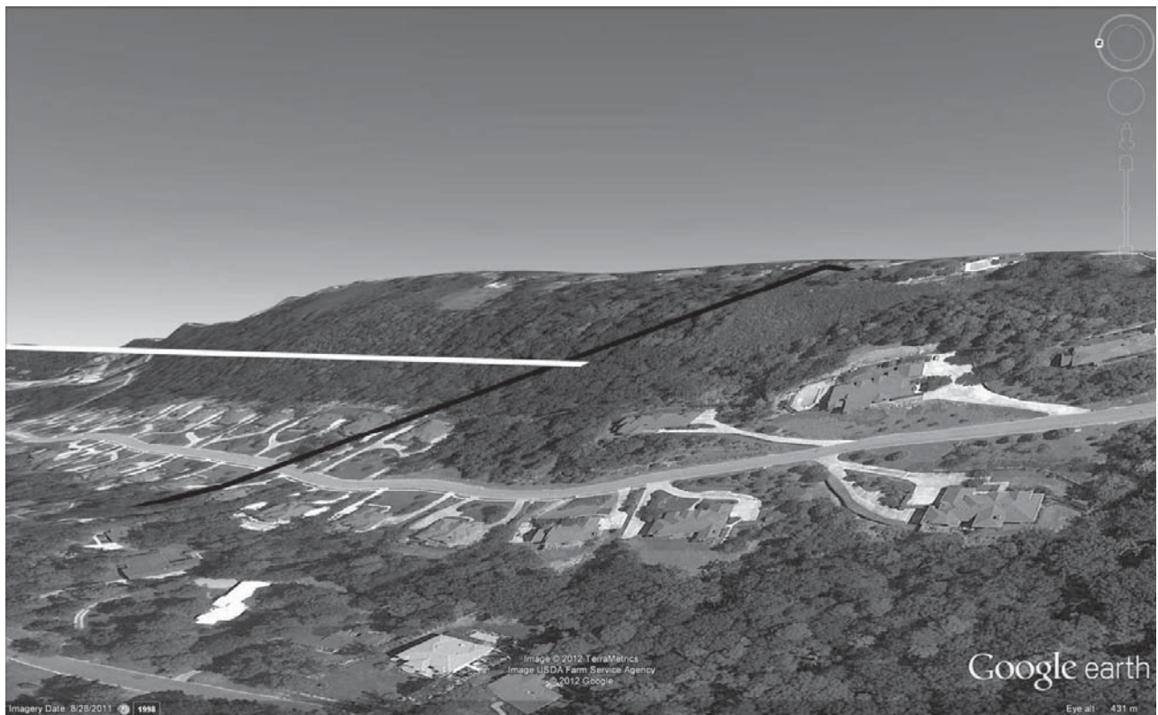
Figure 5 — Tilted view of 23 cm signal path interruption from Example 1 accompanied by Elevation Profile showing signal path drawn from antenna to antenna with cursor pointing to first interruption point.
