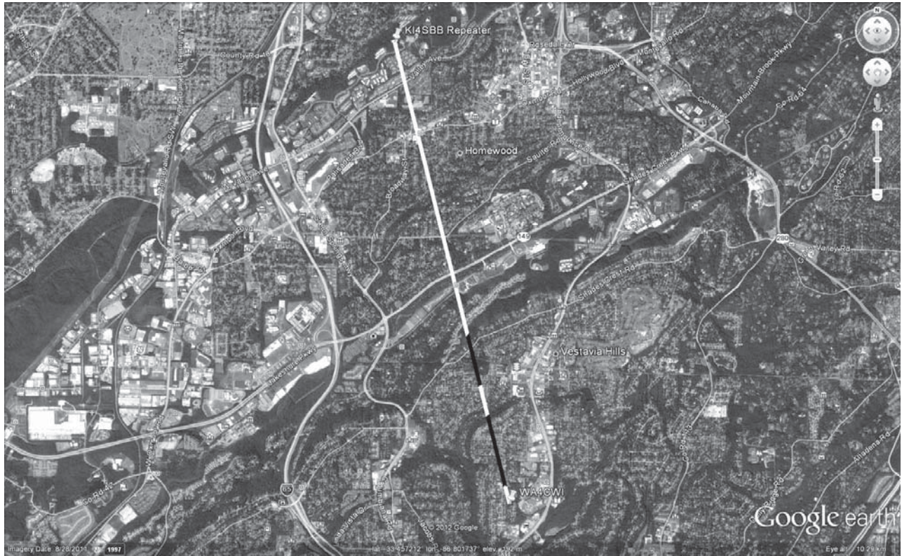
Figure 4 — Four mile 23 cm signal path interrupted twice by terrain peaks from Example 1.
