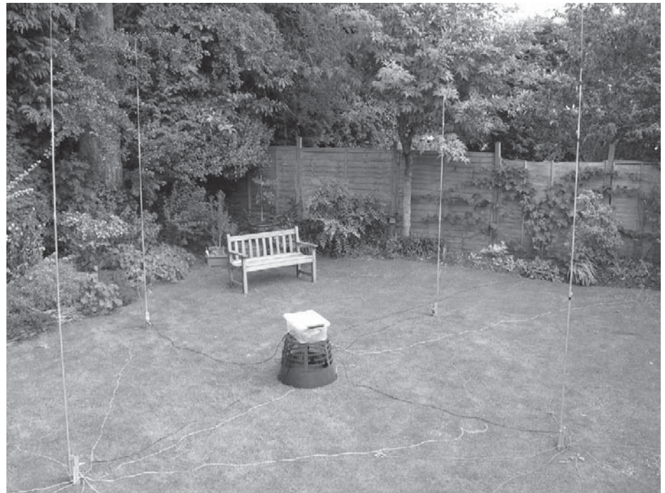
Figure 2 — The disposition of the elements, feeders and sets of eight quarter wavelength radials.
