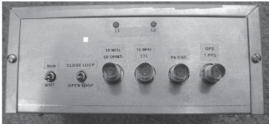
Figure 9 — Here is a photograph showing the front panel of the Rubidium-GPS frequency controller.
