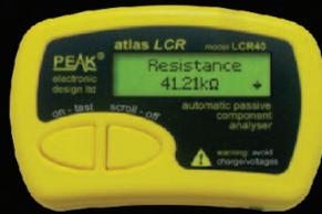
An advanced instrument that greatly simplifies the testing of passive components. Traditional LCR bridges are inherently complex and very time consuming to use. This does everything automatically, it tells you the component type in addition to component value data. What's more, it automatically selects the best signal level and frequency for the component under test.
