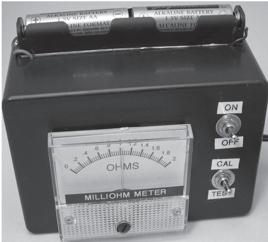
Figure 3 — Here is another view of the completed milliohm meter. The two AA batteries are mounted on the top of the project case.
