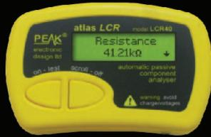
An advanced instrument that greatly simplifies the testing of passive components. Traditional LCR bridges are inherently complex and very time consuming to use. This does everything automatically, it tells you the component type in addition to component value data. What's more, it automatically selects the best signal level and frequency for the component under test.
