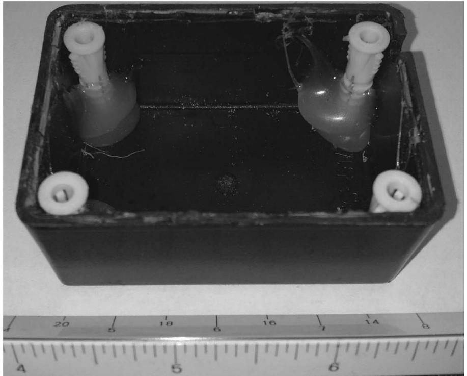
Figure 7 — Here is the empty “RF transparent” wall wart shell that I used to house my Bluetooth module. Note the plastic screw anchors hot glued into the corners to hold the cover screws.
