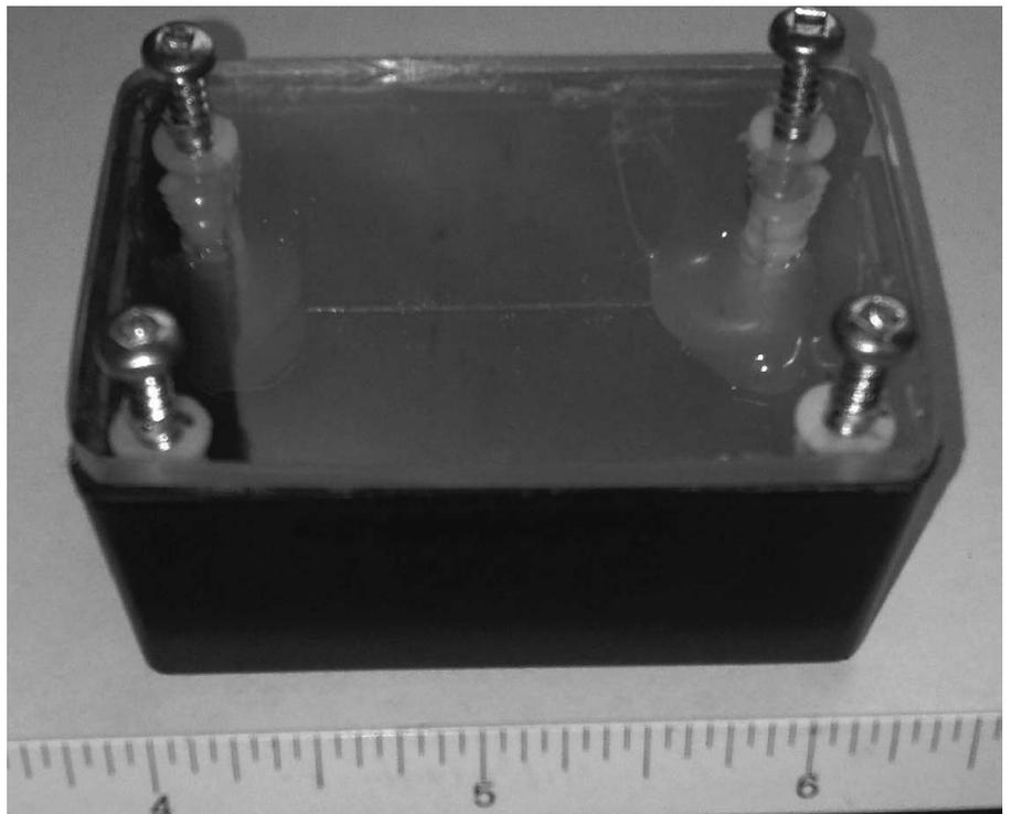
Figure 8 — With a clear plastic cover fastened in place on the wall wart shell, I am able to view the Bluetooth module status LED.
