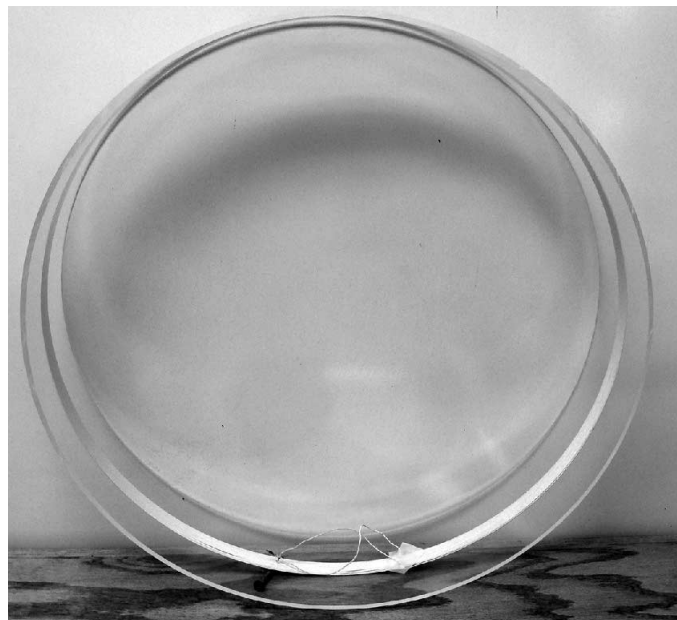
Figure 4 — Photo of 15 inch diameter cast acrylic tubing wound with 18 turns of 175/46 Litz wire.
