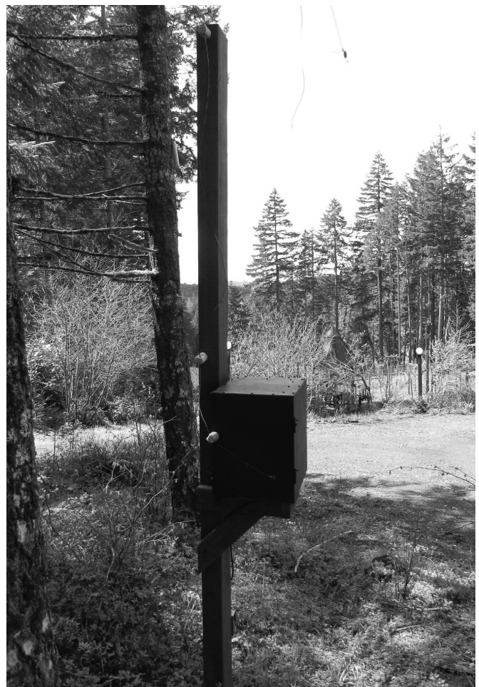
Photo H — Here is the parasitic loop tuning box, which is at the base of the east vertical element. This view is looking west down the low horizontal wire of the loop. The horizontal wire is placed about 15 feet high so delivery trucks and other vehicles can pass under it. The horizontal wire is supported by a tree in back of this view, to achieve the desired height clearance. The insulator is visible in the top left corner of the photograph.
