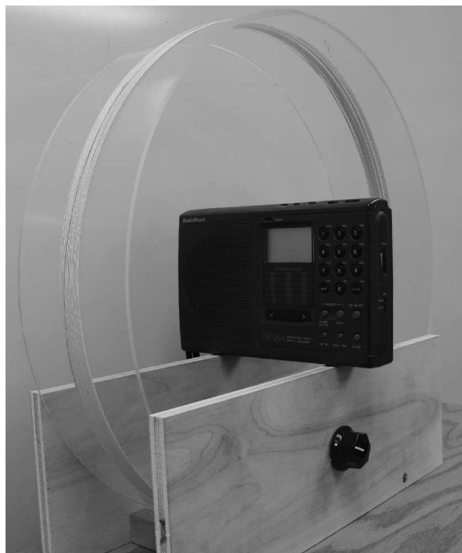
Figure 8 — Example of an external loop antenna combined with a portable medium wave (MW) receiver in order to improve reception of fringe stations.
