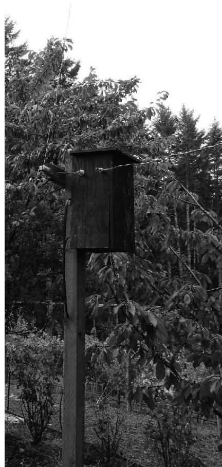
Photo D — The west leg of the driven element: the capacitive boot wire runs to the right.
