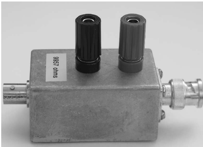
Photo A — This photo shows the assembled shunt impedance adapter. The female BNC connector accepts the signal from the low frequency adapter TX connector. The male BNC connector is the output signal, which goes to the low frequency adapter RX connector.
