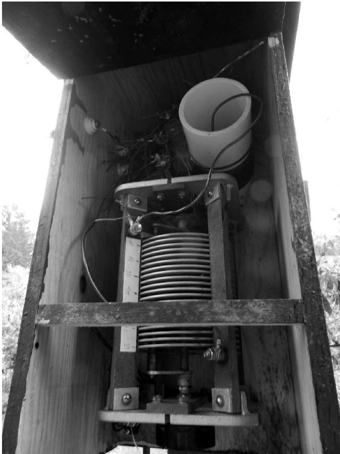
Photo E — The fixed inductor at the west leg. A Russian surplus ceramic switch shorts the inductor out of the circuit when a broadside pattern is desired. The inductor is only used for end-fire patterns.
