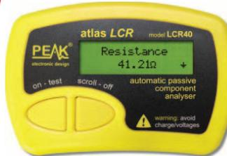
Analyzes coils, capacitors, and resistors.
