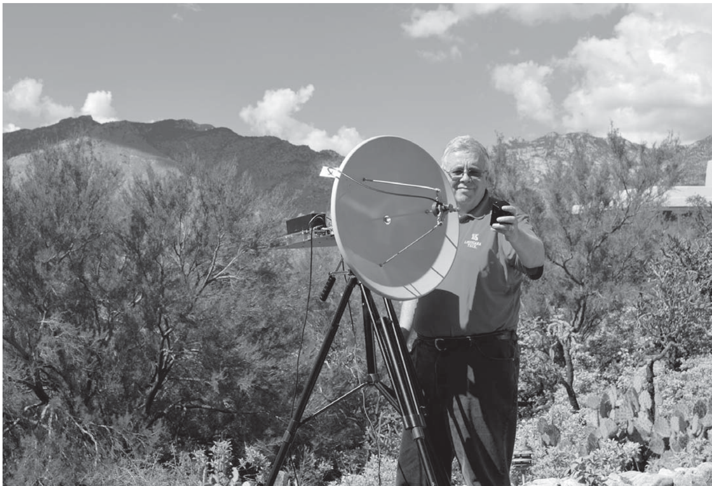
Figure 6 — KI5WL testing his rover antenna with the HB100 based source.
