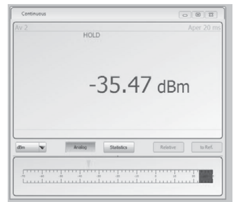
Figure 8 — This screen is a measurement of the signal through the 10.7 MHz filter that was measured in Figures 6 and 7, using a professional broadband power meter.
