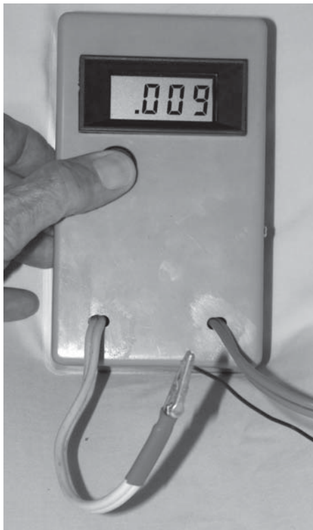
Figure 2 — The author is measuring the resistance of a 4 inch length of #22 AWG copper wire. His thumb is holding down the push-button switch to make the measurement.
