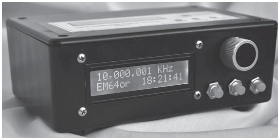
Figure 2 — Here is a completed VFO project, housed in a plastic project box. The Resolution, Band Select, and Reset pushbutton controls are located just below the rotary encoder.
