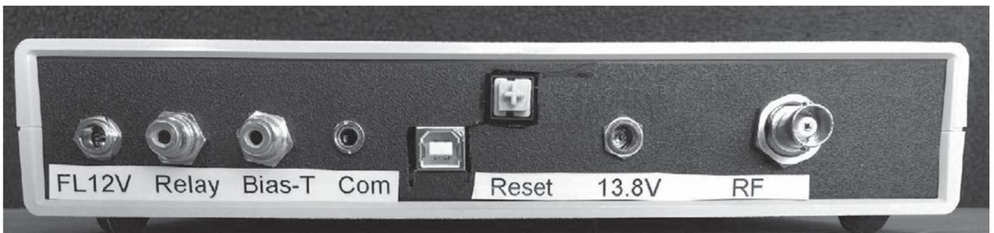
Figure 5 —This photo shows the controller rear panel. The various input and output connections are shown.
