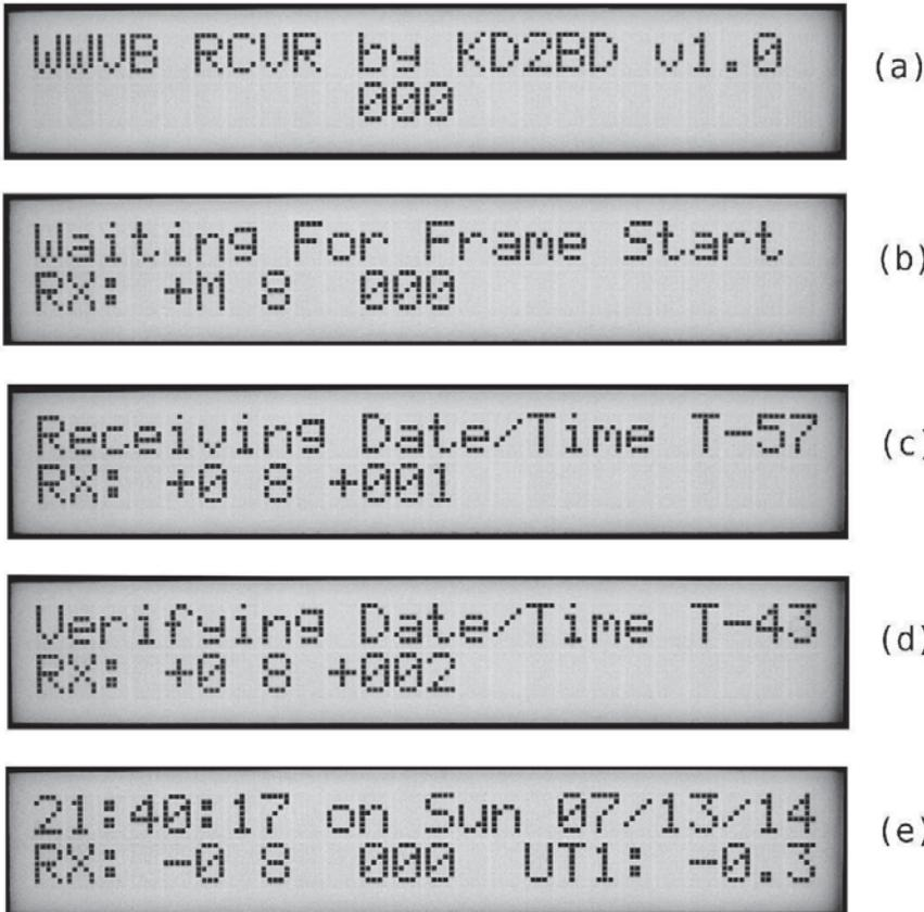
**Figure 17** — These images show the various LCD screens depicting each of the five stages of frequency standard operation following power up. The final stage is where the UTC date and time are continuously displayed and made available to peripheral equipment via the RS-232 port.
