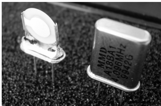
Figure 1 — The internal structure of a quartz crystal unit is shown on the left. The complete package in the metal HC-49U case is shown on the right.
