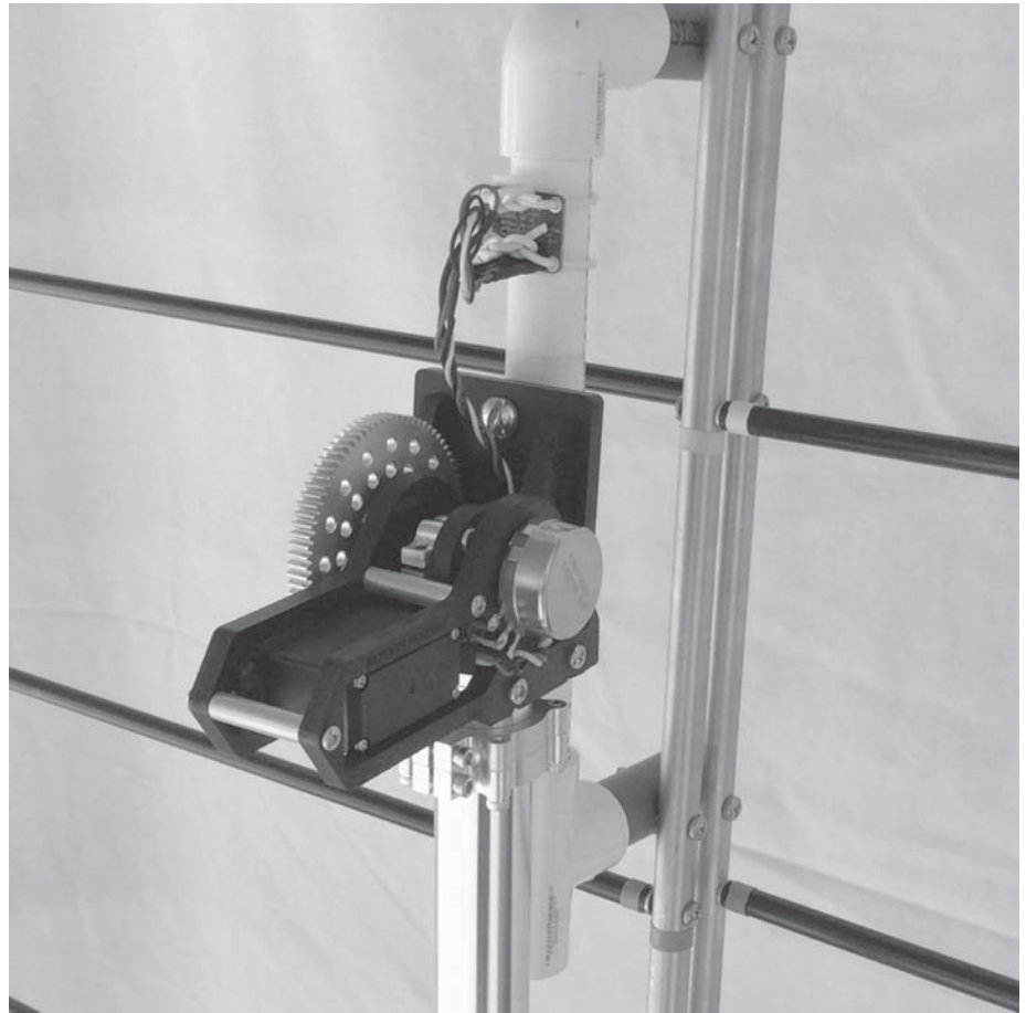
Figure 5 — The elevation gimbal shown with antenna attached.
