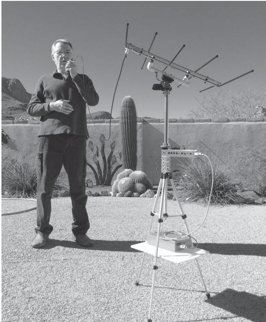
Figure 1 — Tracker gimbal is attached to a tripod and supports an Elk 2m/70cm LPDA antenna.
