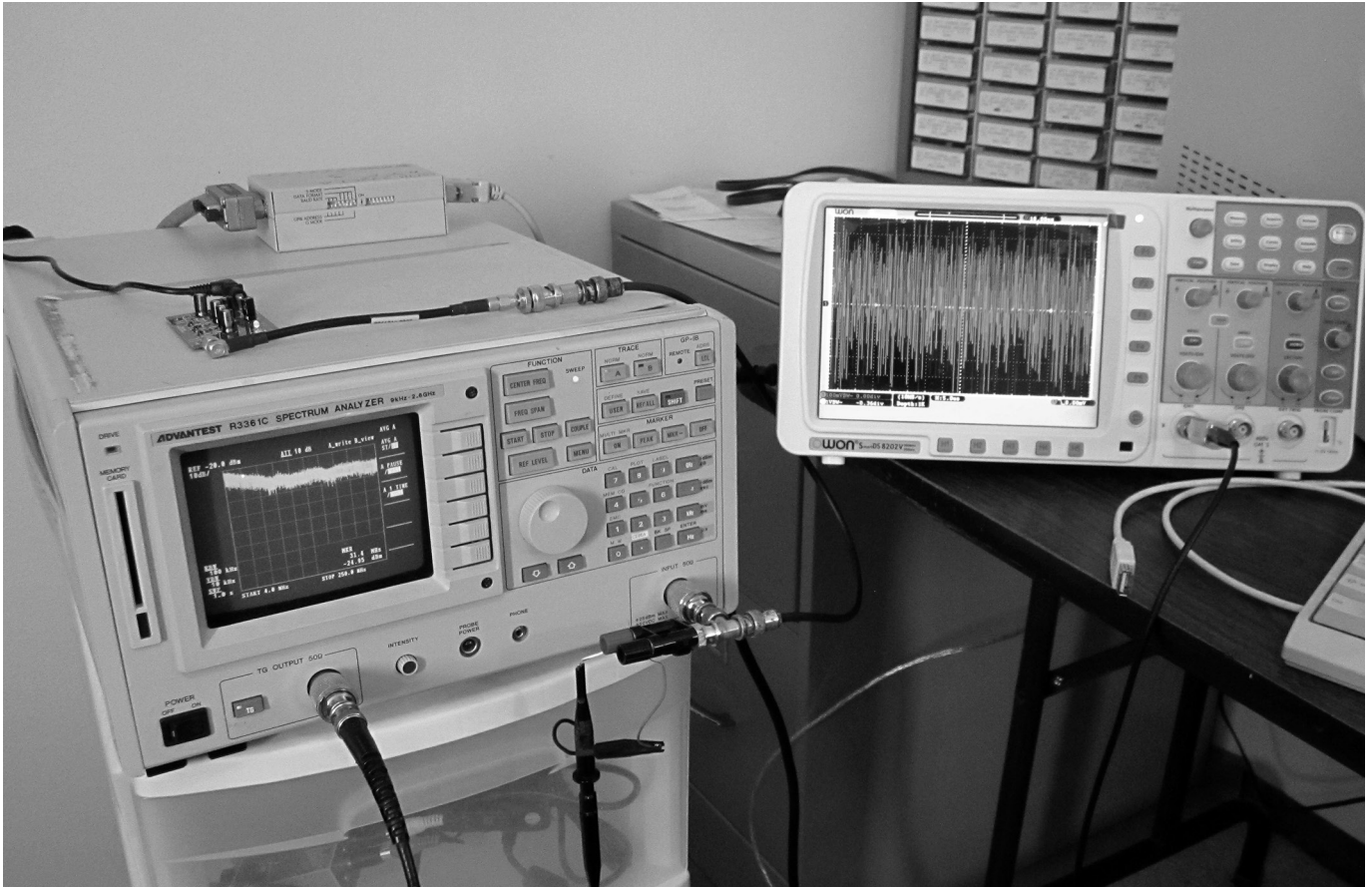
Figure 2 — Spectrum analyzer, oscilloscope and noise source used in this study.
