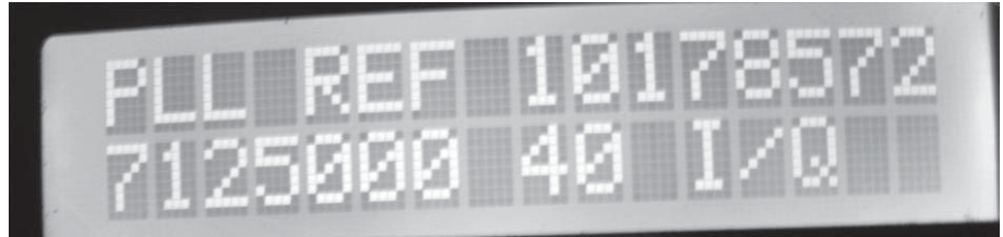
Figure 2 — The LCD shows the PLL reference frequency and the target output frequency.
