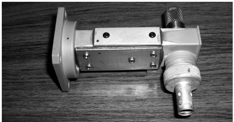
Figure 1 — Using gusset plates to reinforce a waveguide splice.
