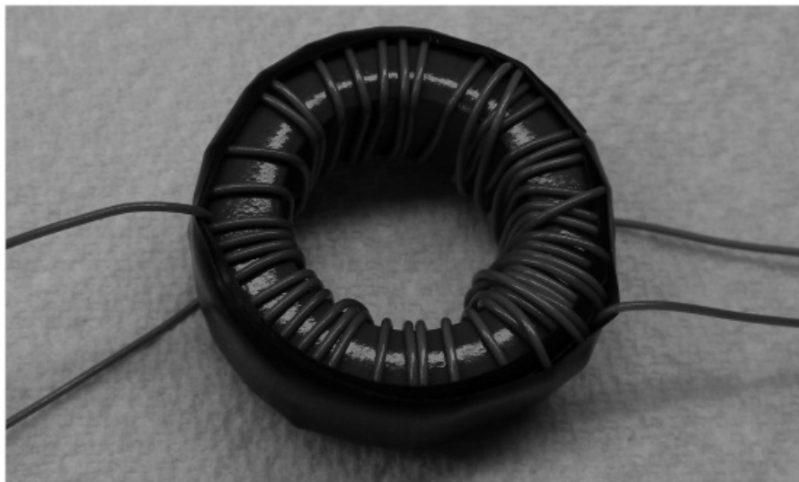
Figure 20 — Primary winding added to the impedance transformer.
