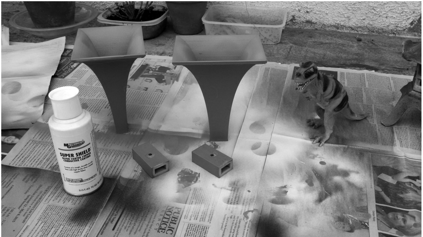
Figure 8 — The four parts were metalized with conductive spray paint, the toy dinosaur shows scale.
