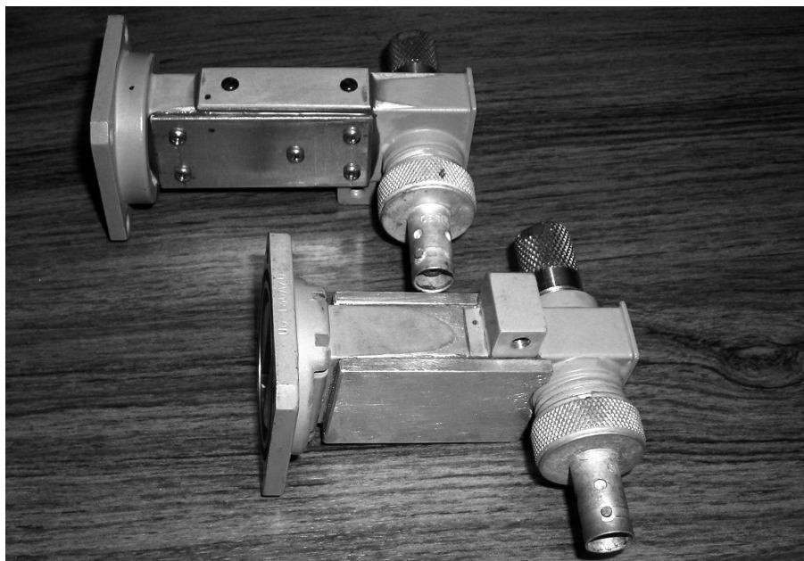
Figure 3 — Completed reinforced waveguide splices.
