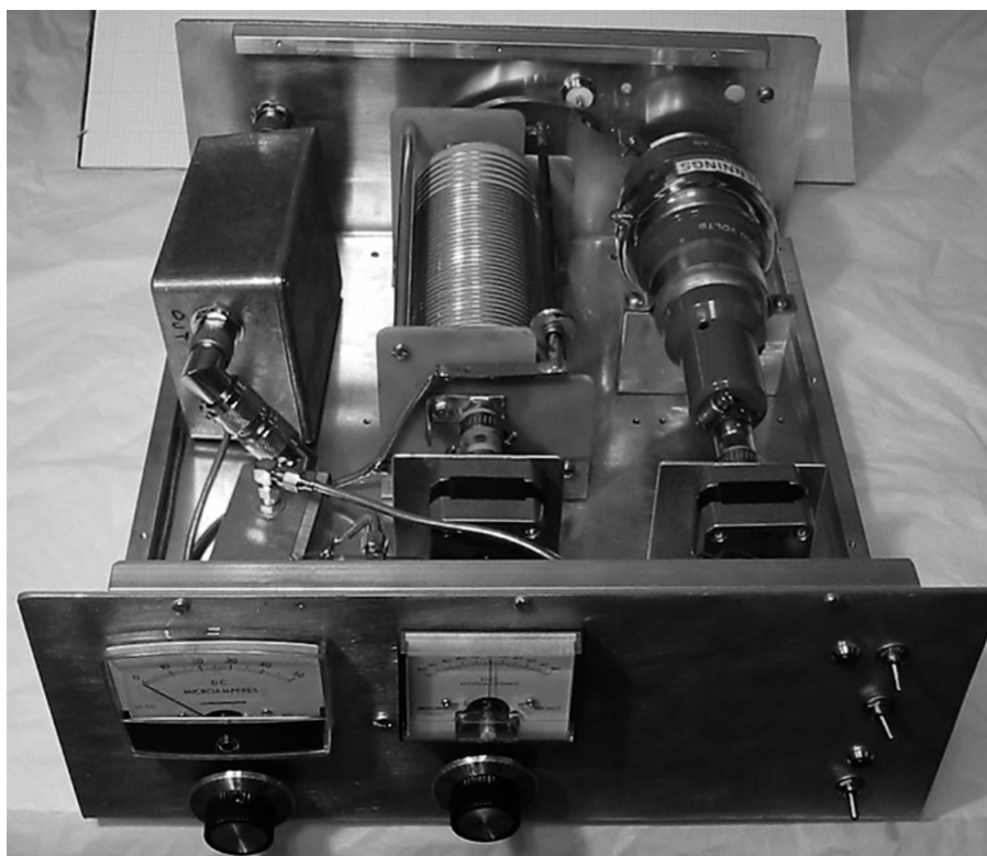
Figure 4 — The L -network matchbox with stepper-driven vacuum capacitor and roller inductor.
