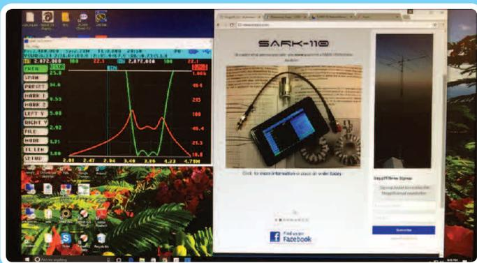
For bench applications, the SARK-110 can be controlled from your desktop computer via the USB interface. Display shows on computer.
