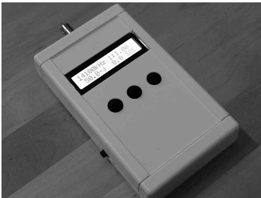
Figure 1 — An image of the DG5MK IV-Meter antenna analyzer.
