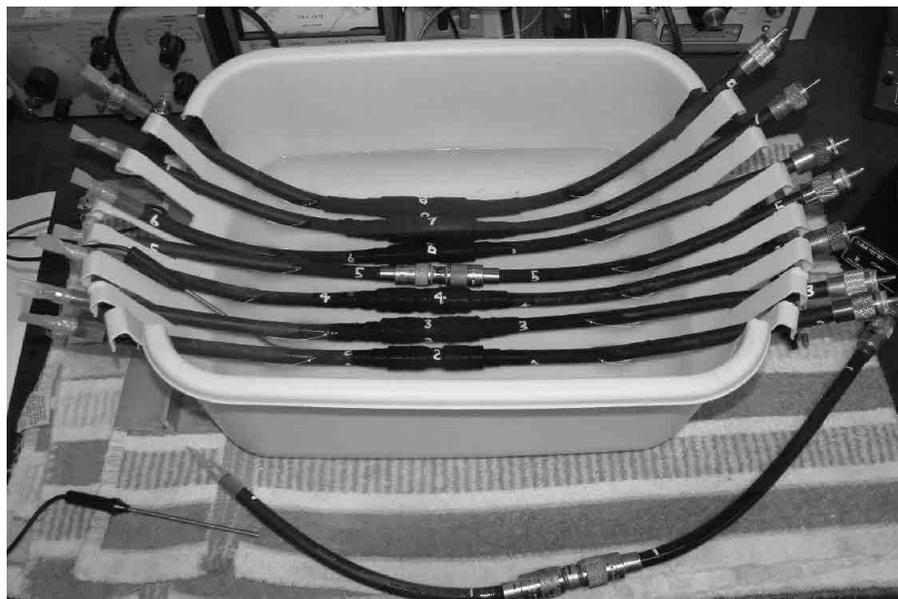
**Figure 2 — The water bath with seven cables immersed, and one dry reference cable.**
