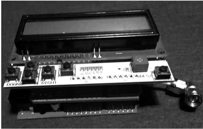
Figure 3 — A 40 MHz frequency generator in two shields: RedBoard (bottom), proto shield with DDS unit (middle), and 20x2 LCD display (top).
