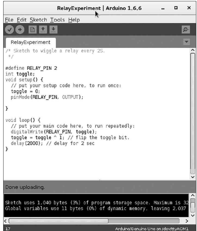
Figure 4 — Arduino sketch to toggle a relay coil on and off at 2 second intervals.
