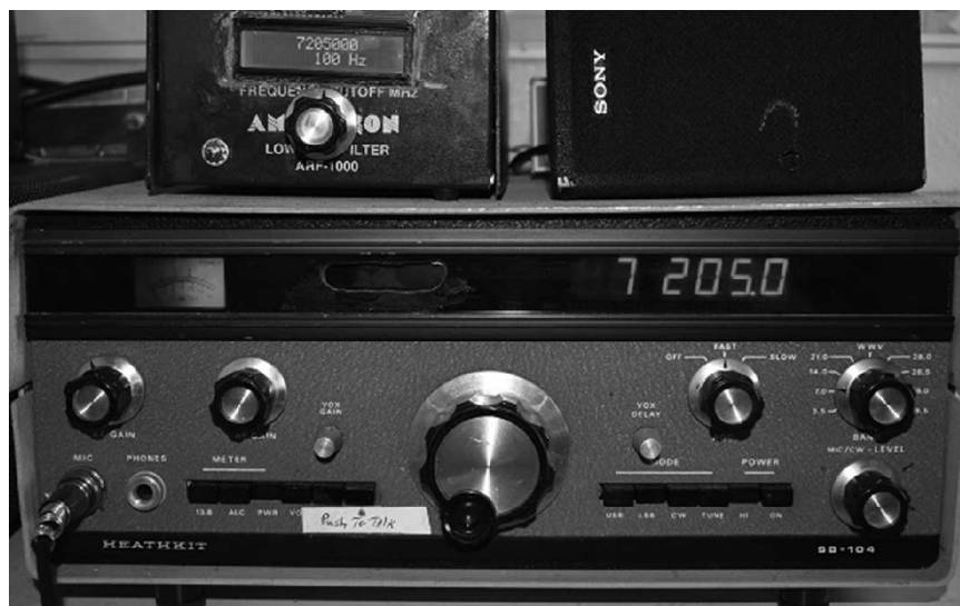
Figure 4 — The Arduino-based external VFO is on top of the Heathkit SB-104 transceiver. [Tom Sowden, W6KAN, photo.]
