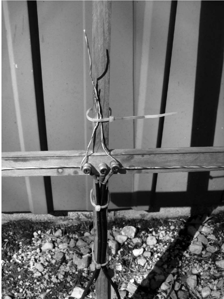
Figure A2 — Feed system via 50 to 200 \Omega balun for 144 MHz three-high stack of square loops antenna.
