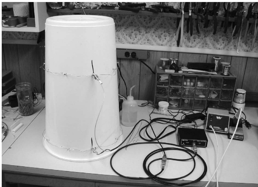
Figure 2 — Calibration test fixture shows the AIM4170 as the VNA, but the same fixture was used to calibrate the N2PK vector network analyzer that was used for the actual measurements.
