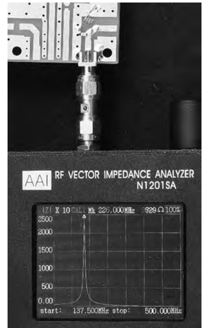
Figure 11 — Measuring resonant frequency of a parallel-resonant circuit to determine the value of a small inductance.
