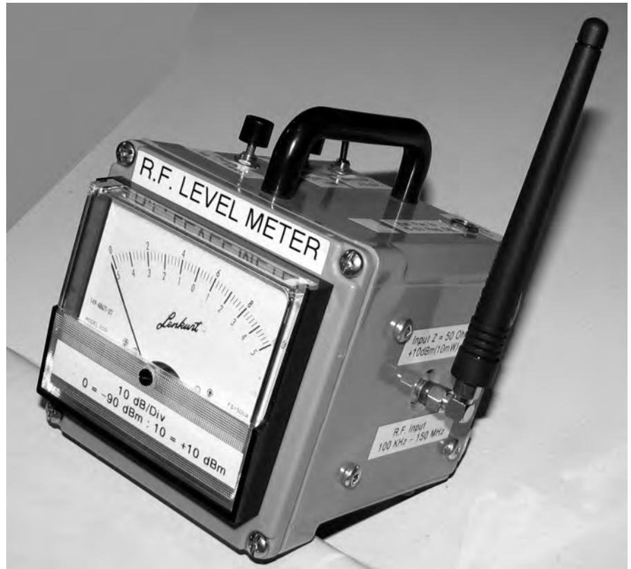
Figure 6 — Field strength meter housed in a 4-inch cube junction box.
