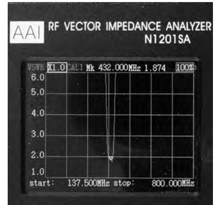
Figure 13 — Input VSWR of a band-pass filter with 50\ \Omega termination on the output showing the filter frequency range.
