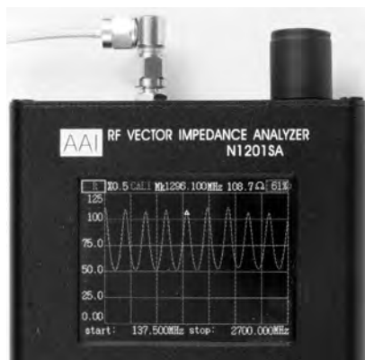
Figure 6 — Swept frequency plot of R , for calculating cable characteristic impedance.
