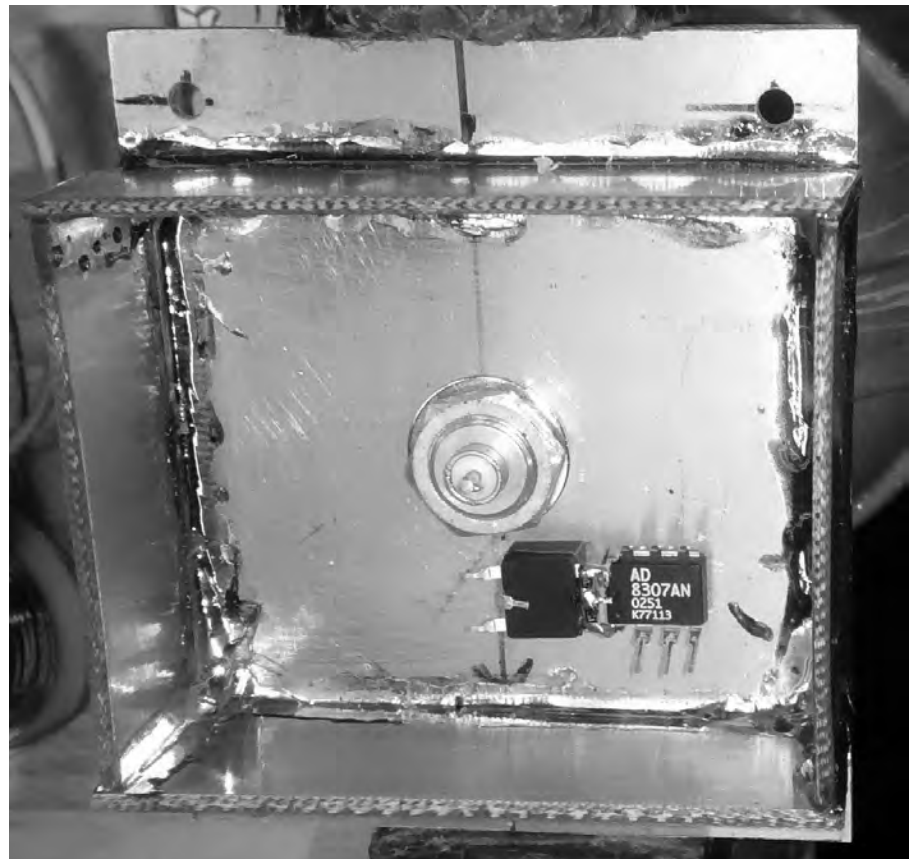
Figure 7 — “Dead bug” mounting style of the AD8307 RF detector, and the 1:16 wideband step-up transformer.
