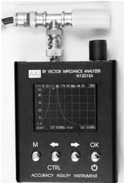
Figure 8 — Measuring resonant frequency of a stub
