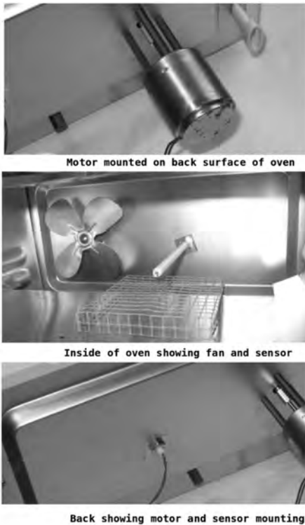
Figure 5 — The motor mounted on the back surface of the oven (top image), an inside view showing the fan and the temperature sensor (middle image) and an outside back view of the assembly (bottom image) showing the motor and sensor mounting.
