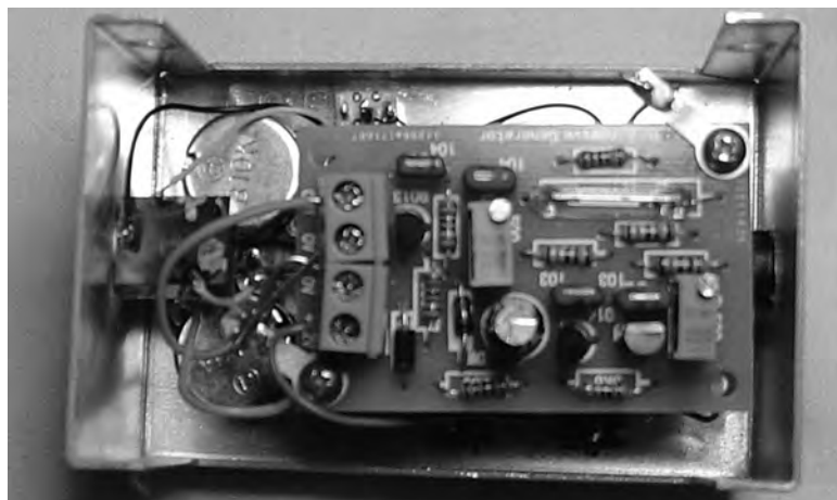
Figure 6 — Internal view of the oscillators mounted in an aluminum box.
