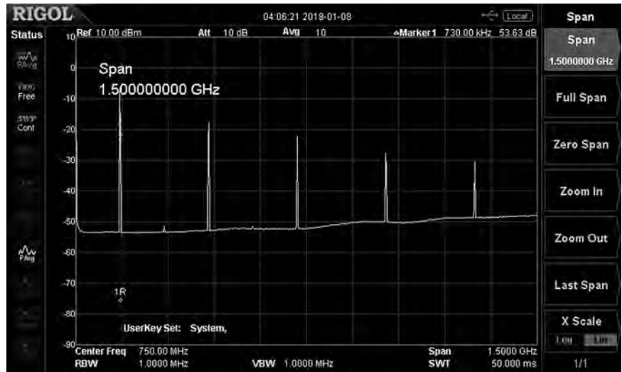
Figure 7 — Spectrum analyzer plot of USB 2000 Hz tone at 144.270 MHz, full span of 1.5 GHz.
