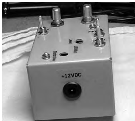
Figure 10 — The dc input power connector is on the side of the box.
