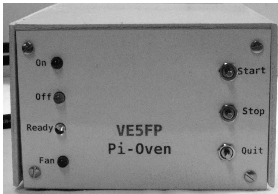
Figure 10 — Front panel of the Pi-Oven controller. Push Start to begin the solder-reflow process.
