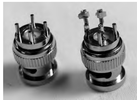
Figure 11 — Photo showing small BNC adapter on the left and, on the right, the added contacts for measuring crystal parameters.
