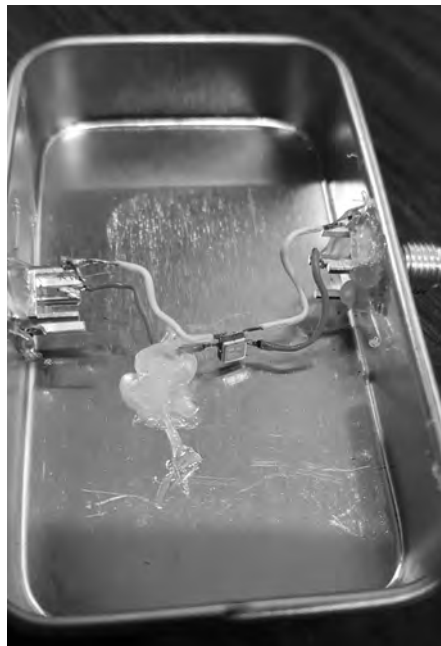
Figure 3 — Prototype filter in a tin housing.
