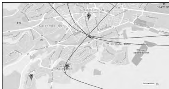
Figure 11 — Localization of an unknown signal at 391 MHz (approximately 12 kHz bandwidth). The measured position is located near the local post office and the train station.
