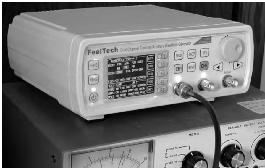
Figure 1 — Photo of FY6600 dual channel function, arbitrary waveform generator used in this project.
