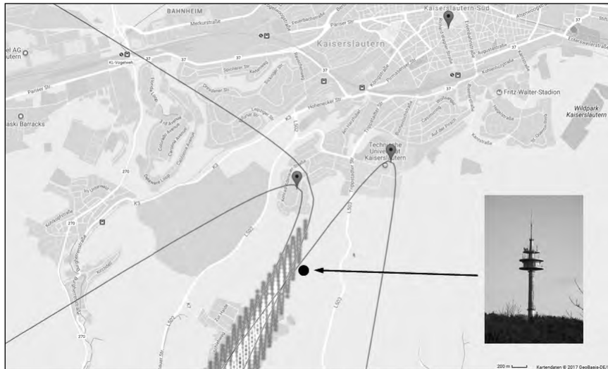
Figure 12 — Localization of a FM broadcast signal at 96.9 MHz, where the transmitter is located to the side.
