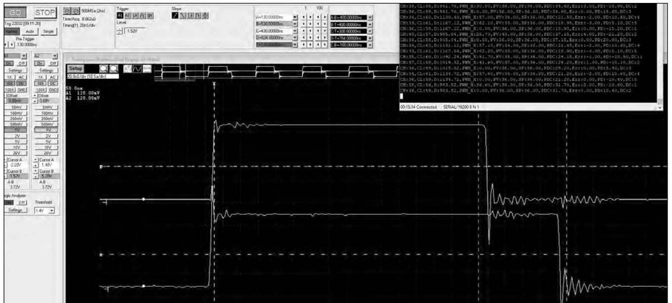
Figure 16 — The upper trace is the logical AND of the bottom trace with the 10 MHz OCXO.
