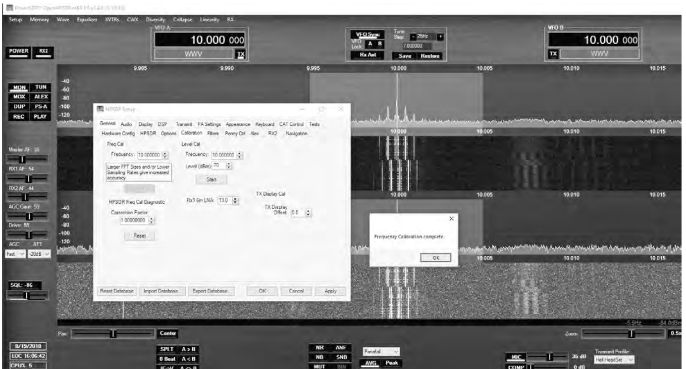
Figure 11 — The results after using the Themis GPSDO as the 10 MHz clock input.
