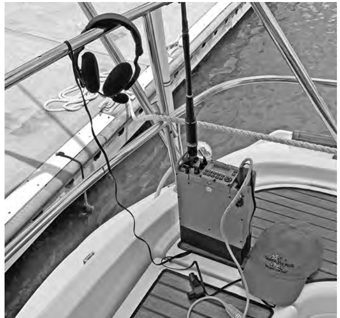
Figure 15 — Portable installation of a Rohde & Schwartz M3TR transceiver, ready for Amateur Radio contacts from a boat. [N1UL photo]
